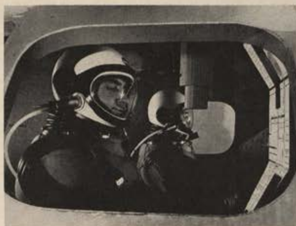
Technicians from NASA Marshall Space Flight Center, Ala., and Hayes International Co., Huntsville, Ala., wearing Apollo-type space suits, test mockup of Lunar Mobile Lab (MOLAB) at Lockheed plant in Sunnyvale, Calif. MOLAB would allow two-week moon survey.
