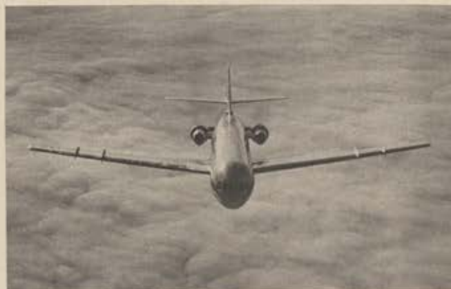
Shown flying over the clouds is a prototype of the Super Caravelle, powered by two GE CJ805-23C jet engines. It is a refined version of the short- to medium-range Caravelle.
