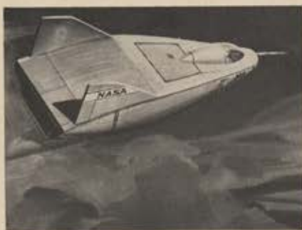
Forerunner of shuttle vehicle to supply orbiting spacecraft, Northrop M-2 is sketched as it would appear from B-52 mother ship in glide tests to begin soon at Edwards AFB, Calif.
