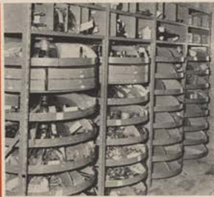
Sometimes it takes longer to find a part than it did to procure it. The streamlined, revolving storage bins (right) should help in this regard.
