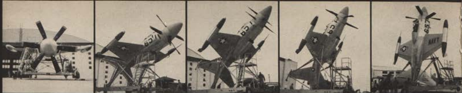
SPECIAL CRADLE LIFTS XFV-1 from prone position (for servicing) to upright for vertical takeoff.
