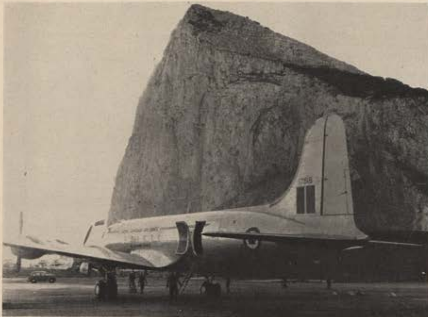
RCAF transport operations cover the globe. Here a North Star transport of the 412th Squadron stops off at Gibraltar. The North Star, Canadian-built adaptation of the DC-4, is powered by four Rolls Royce Merlin in-line engines.
