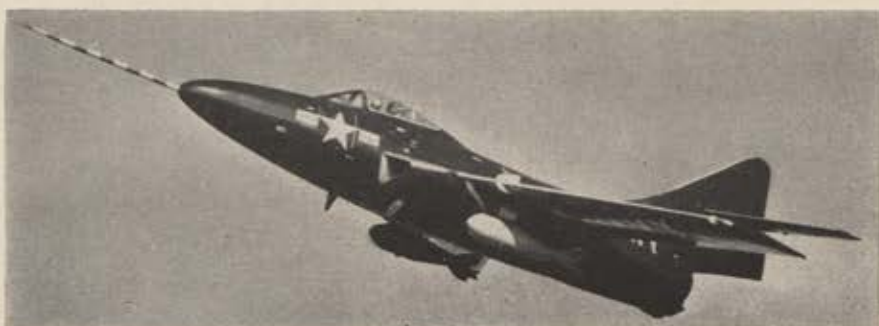
The Grumman F9F-6 Cougar, Navy's first sweptwing jet in squadron service, shown toting two 1,000-lb. bombs. The Cougar also has four 20 mm cannon.
