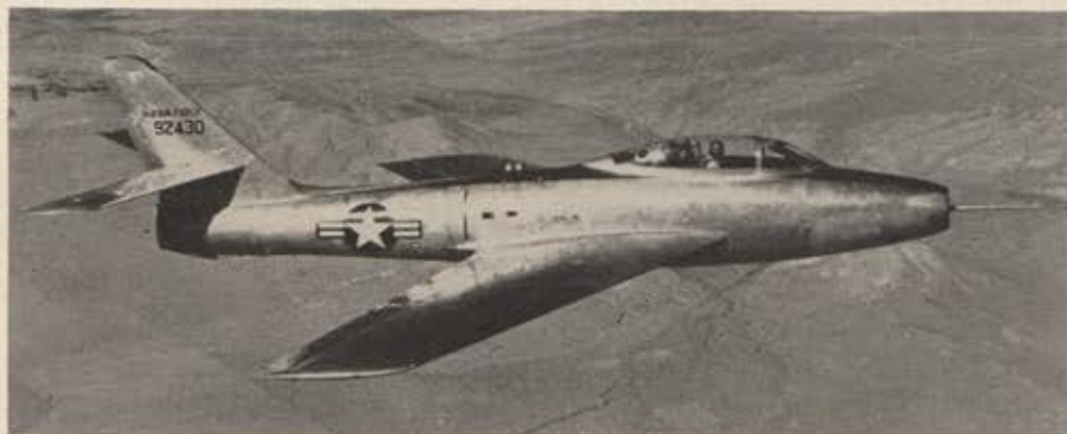
Dual-mission plane. Republic's F-84F, designed as fighter-bomber, is fast enough to be escort or interceptor.
