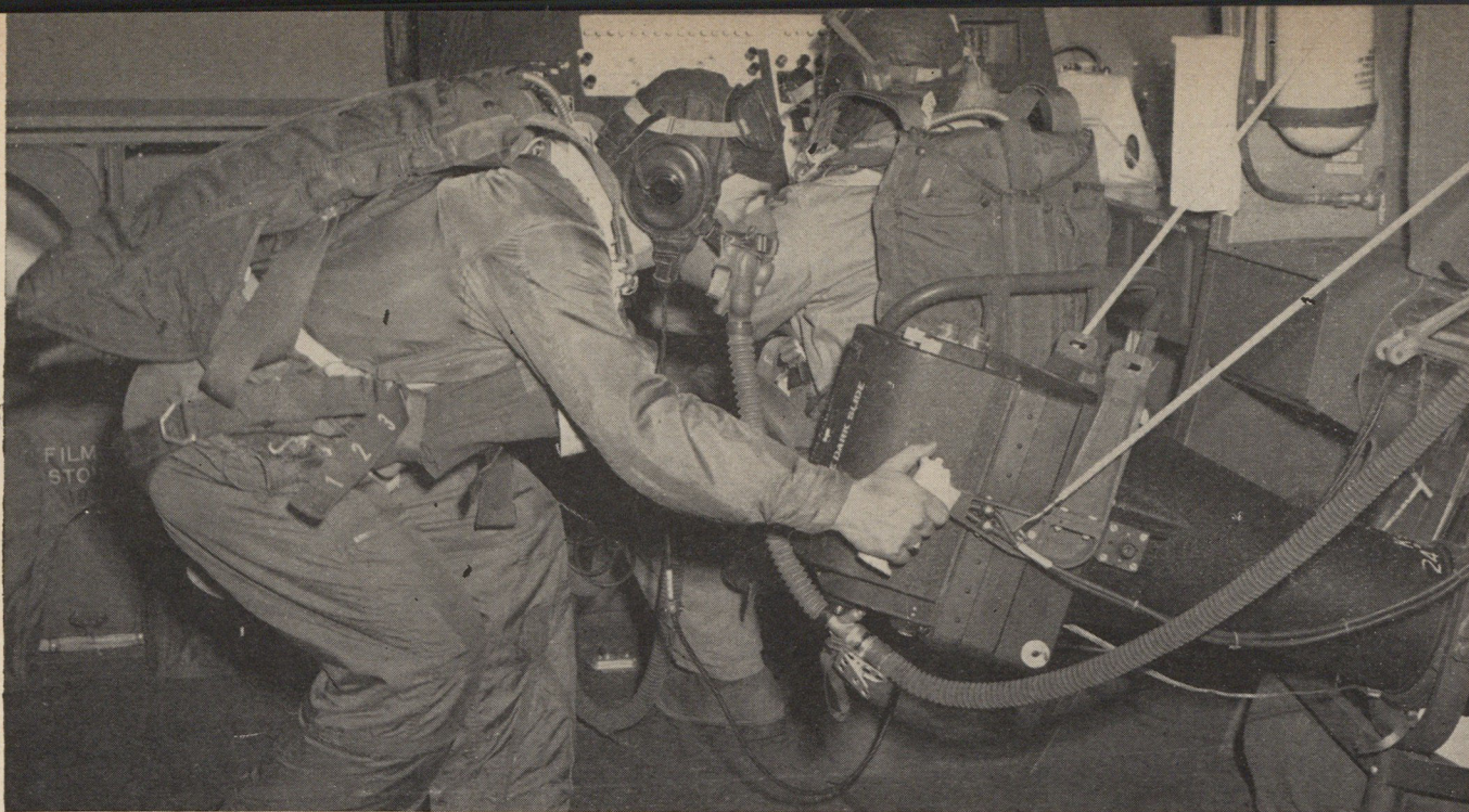
An airfield lying ten miles off the flight path of the RB-36 is picked up by the lens of this king-size oblique camera.
