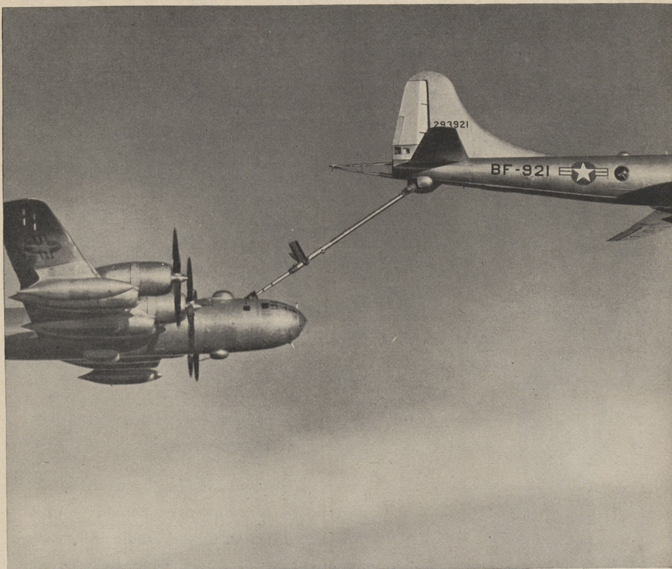
With airplane-like controls, operator in tail of B-29 tanker "flies" telescoping gasoline boom into slot on nose of B-50 receiver plane.
