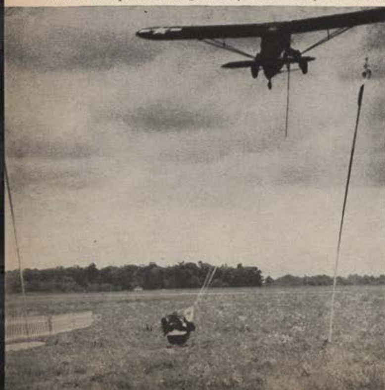
AAF's human pick-up system permits rescue of men in inaccessible terrain and behind enemy lines. Low-flying plane hooks nylon loop, picks up man with less strain than a parachute jump. This photo shows man pulled from ground by means of special harness.
