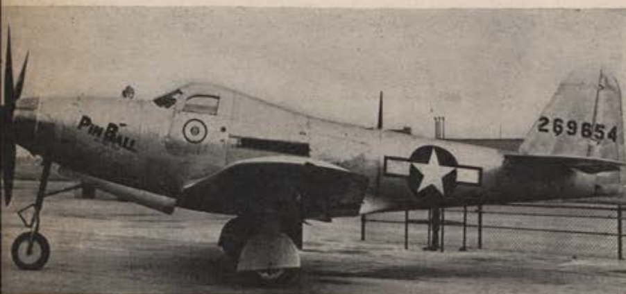
"Pinball," the P-63 target plane shown above, blinks in pleasure when gunnery trainee pots it with frangible bullets. This recent addition to AAF's training program enables gunners to perfect their technique under simulated combat conditions.
