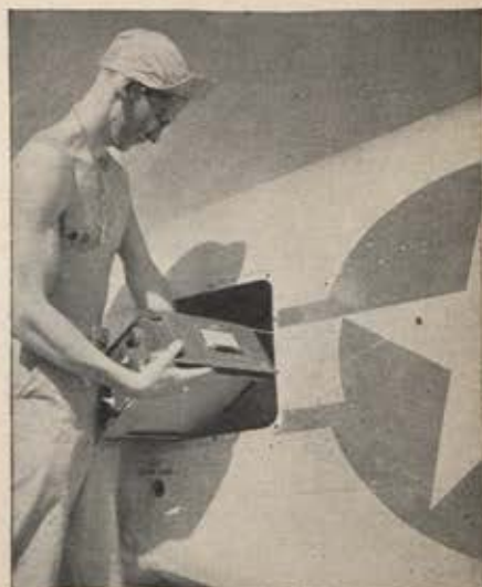
Camera specialist is here shown changing a magazine on an aerial camera used on a P-51.
