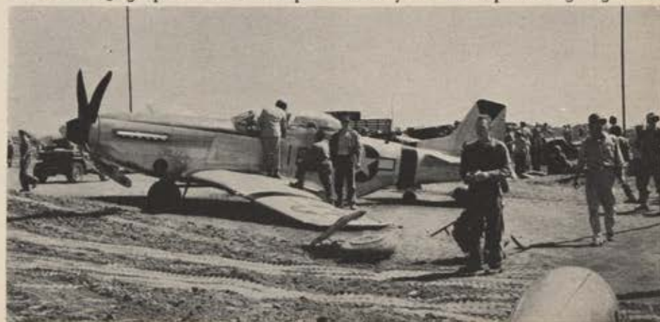
The second P-51 to land at Iwo hit a soft spot in the airstrip. Mechs start repairing damage.
