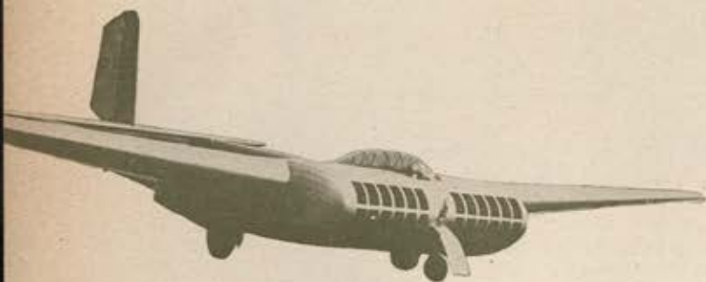
CG-16 Glider giant , shown below and at left above, has twin-boom construction with cargo compartments forming part of wing. CG-10A, at right above, can load six tons of aerial freight through split doors in fuselage rear.
