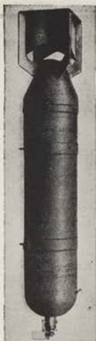
At right is the photo flash bomb used for night aerial photography. At the peak of the flash, it provides about one billion candlepower. Above is a close-up of the bomb's fuse head.
