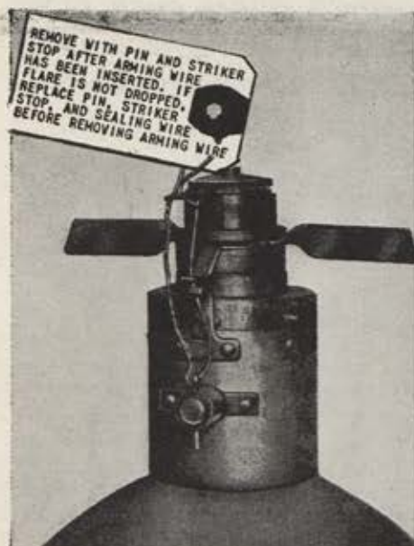
At right is the photo flash bomb used for night aerial photography. At the peak of the flash, it provides about one billion candlepower. Above is a close-up of the bomb's fuse head.
