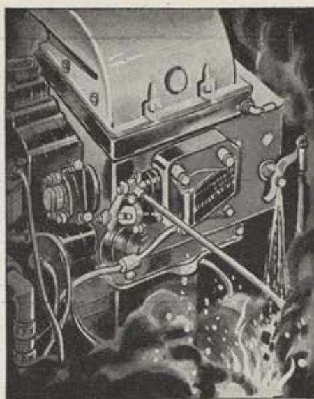
If gasoline is permitted to escape from a loose connection, fire is sure to result.
