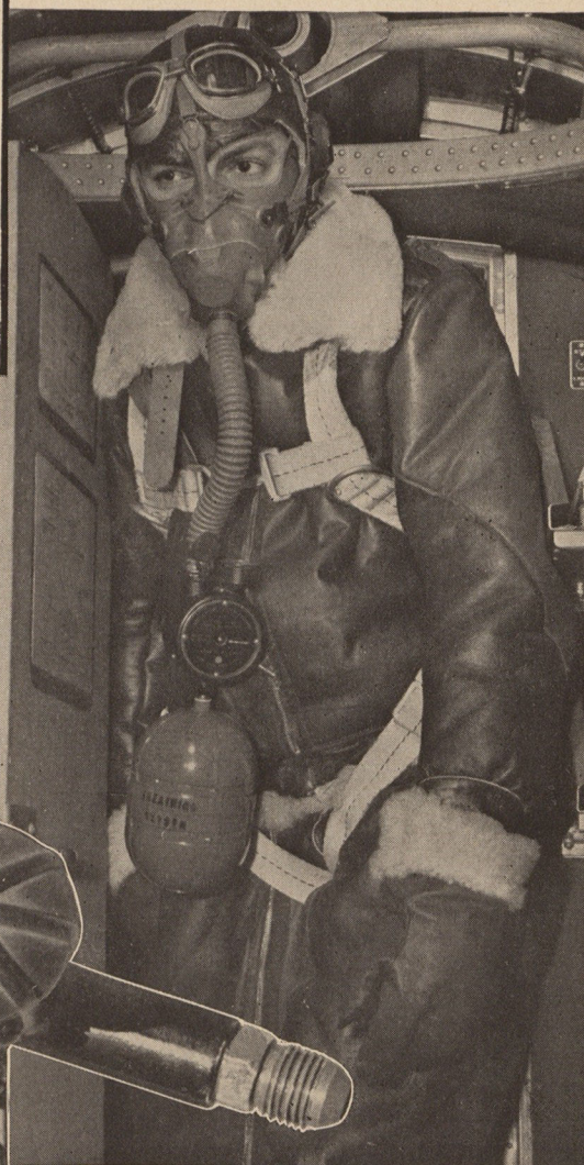
5. This crew member displays good sense by using the portable oxygen unit, known as the walk-around bottle, while moving about in a plane at high altitude. The equipment is used with the A-10 mask and provides a 4- to 8-minute supply of oxygen, depending on the altitude and the activity of the user.
