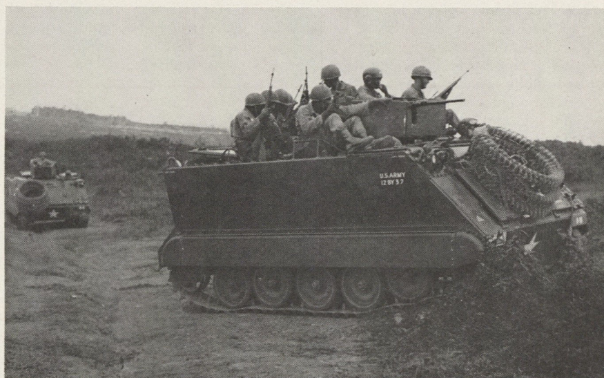
M-113 armored personnel carrier is often employed in Vietnam in role of infantry-accompanying tank. It has been modified by adding more machine guns, recoilless rifles, or 81-mm mortars. Heavy Viet Cong weapons can hurt it, but are seldom encountered.
