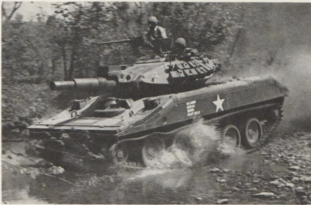
Cadillac-built General Sheridan armed reconnaissance vehicle is entering operational service in June. Its 152-mm gun-launcher fires conventional rounds or the new Shillelagh guided missile.
