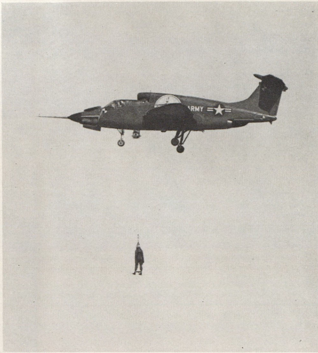
Possibility of rescuing downed pilot by lowering cable from hovering V/STOL aircraft is demonstrated by XV-5A, shown here winching in a 235-pound (106 kg) dummy. XV-5A, built by Ryan Aeronautical Company, employs General Electric lift-fan design.
