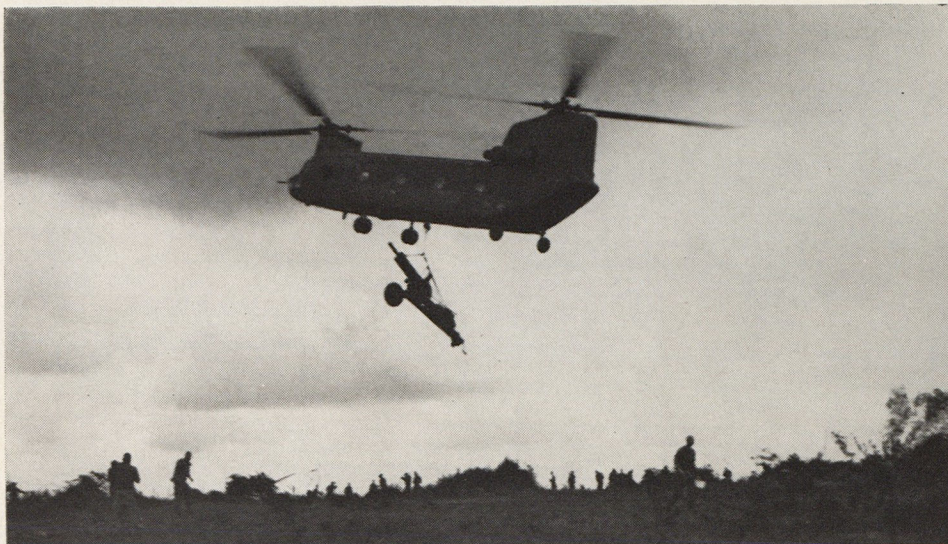
Modern method of moving artillery pieces is demonstrated by this Boeing Vertol CH-47 Chinook of 1st Cavalry Division as it lifts 105-mm howitzer to new location. Helicopters can readily concentrate firepower, even on hilltops inaccessible by road, to smash an enemy concentration, and disperse it again as soon as the action is over.
