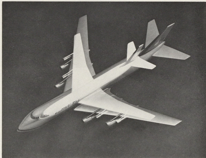
Size of new Boeing 747 jetliner in comparison with present 707-320 Intercontinental is shown in this double exposure. The 707, largest airliner now in service, is 152 feet (46.3 m) long, with 145-foot (44.2 m) wingspan. It weighs 164 tons (148.7 mt) fully loaded, carrying up to 199 passengers. In contrast, new Boeing 747 is 228 feet (69.5 m) long, with wingspan of 195 feet (59.4 m). It will weigh 340 tons (308.4 mt), carrying 490 passengers. First order for 25 747s was placed by Pan American World Airways.
