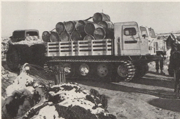
U.S. Army is testing RN110 track-truck, built by Nodwell in Canada, for Arctic operation. Powered by 6-cylinder diesel engine, it will traverse snow and tundra at 12 mph (19 km/hr).
