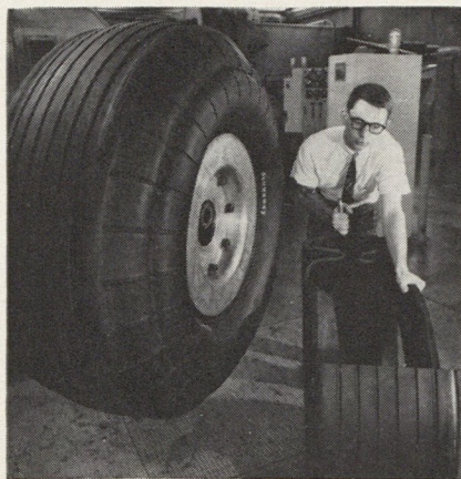
Future aircraft may employ B. F. Goodrich self-folding tire which occupies one-half to three-fourths the space of conventional tire during flight, but inflates to full size, left, for takeoff and landing.
