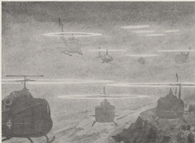
Formation flying. Pilot "sees" other aircraft by means of radar beacons mounted on the blades of other helicopters in the formation.
