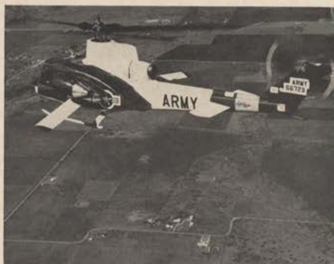
Record-breaking rotorcraft speed of 250 mph was logged by this Bell compound helicopter, basically a UH-1B modified by adding stubby wings and pair of J69 turbojet engines.
