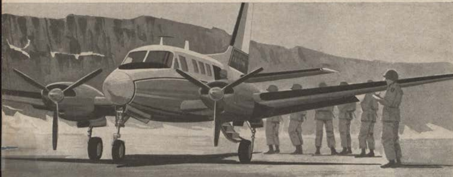
2. Two 380 hp Lycoming supercharged fuel injection engines power this U-8 to speeds of 252 mph.
