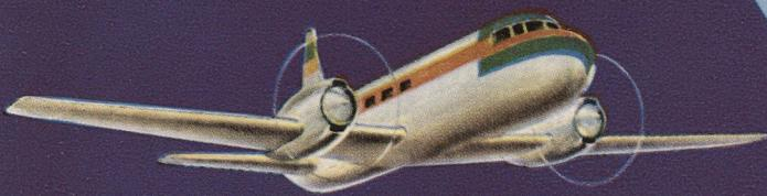
The sturdy and efficient Convair-Liner airframe has demonstrated complete adaptability to the installation of gas-turbine power plants. America's first turboprop transport, the Allison Convair-Turboliner, already has accomplished a series of successful test flights.
