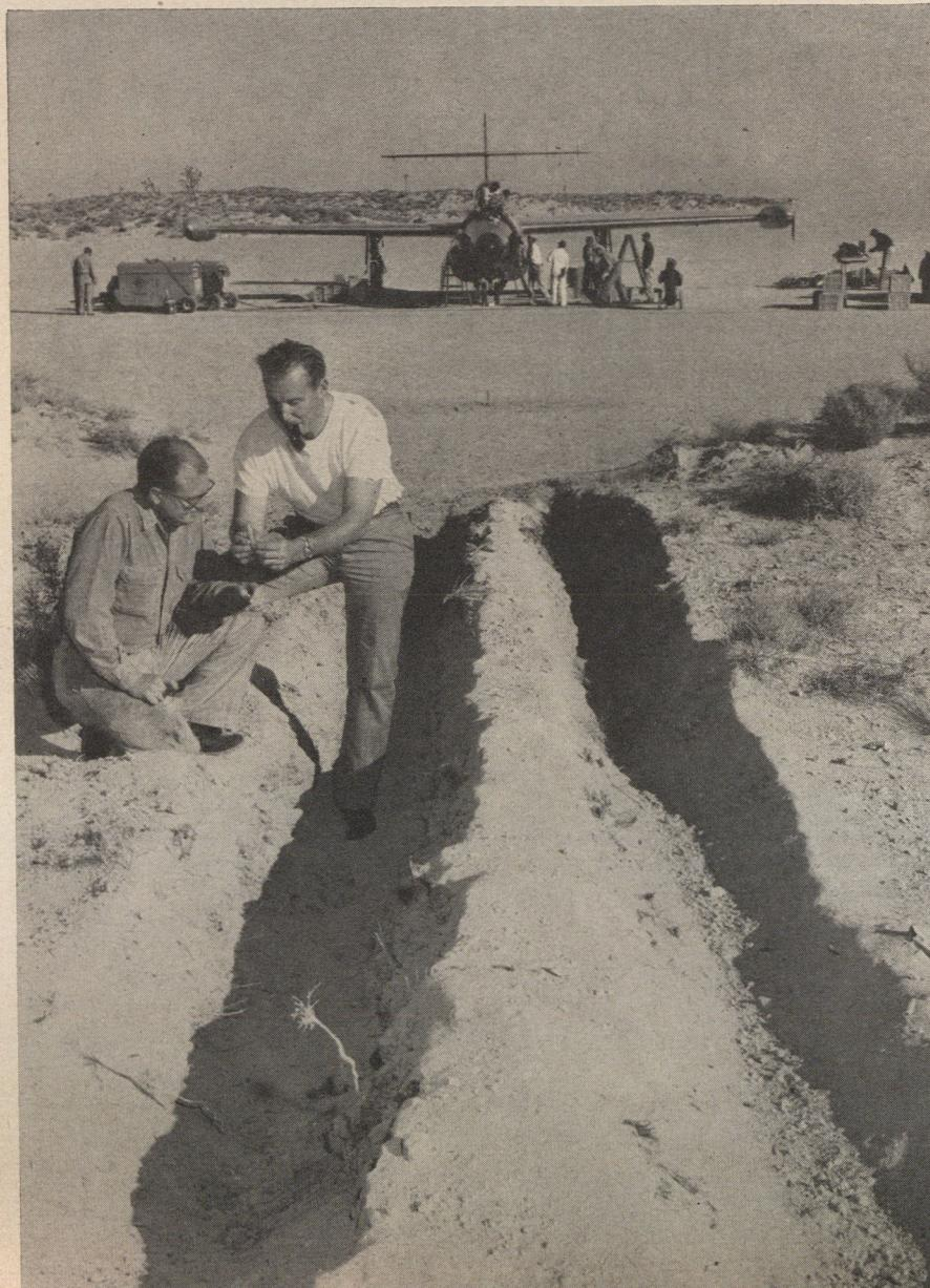
The Scorpion packs a potent sting. Six 20-mm cannon in F-89's nose dug these deep trenches during firing tests on the California desert near Edwards Air Force Base, Muroc.
