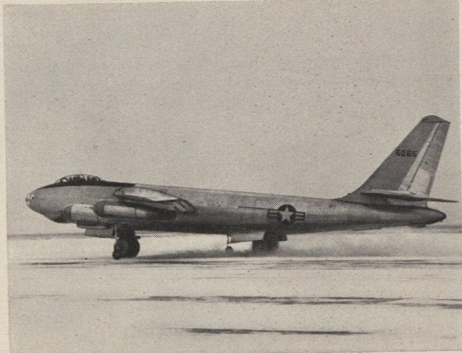
**SAFE STOPS.** Boeing has designed and built a new aircraft braking device, adopted by the Air Force for certain types of planes. Self-activating, this mechanism permits the application of full brake power with no skidding or wheel-locking on wet or icy runways.
