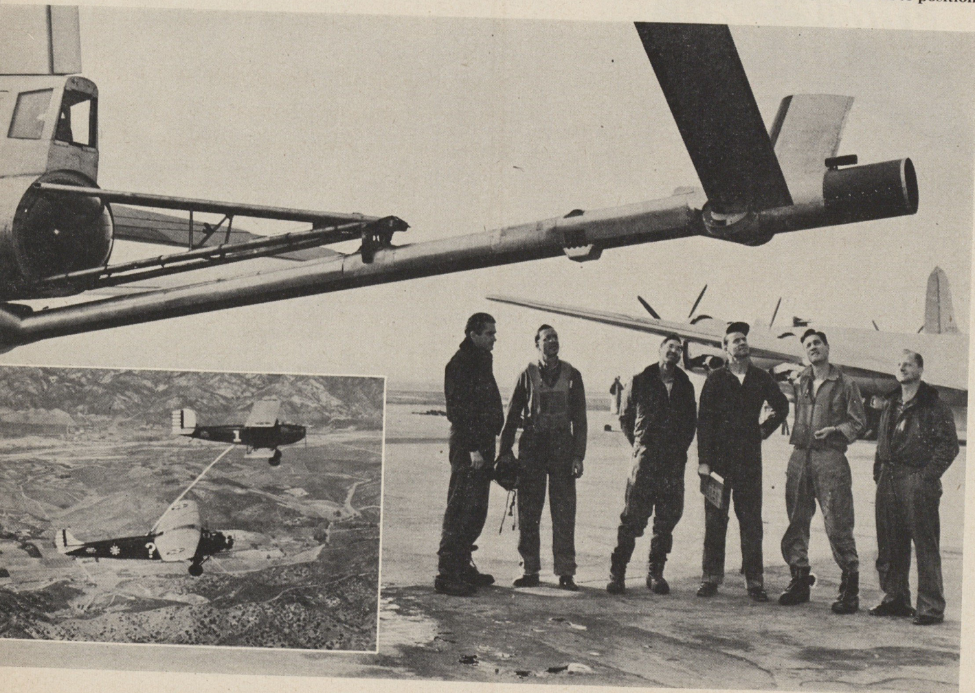
Today's flying boom for air-to-air refueling is a far cry from the ordinary filling station hose used in early attempts like that of the Question Mark in 1927, lower inset. Developed by the Boeing Aircraft Company, the boom makes it possible to refuel in flight with greater speed and at higher altitudes than previously was possible. "Clancy" in the tail, above left, "flies" the boom into position for coupling. Upper right, a B-50 gasses up. Note "vanes" which guide boom to position.
