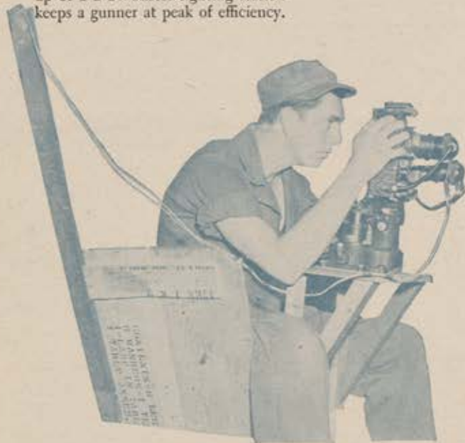
Frequent practice with this mock-up of a B-29 blister sighting station keeps a gunner at peak of efficiency.
