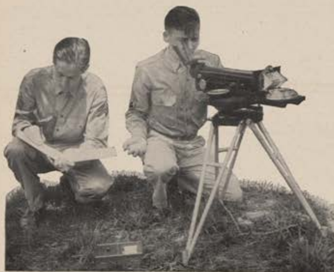
Geodets use an equiangulator to get their longitude and latitude.
