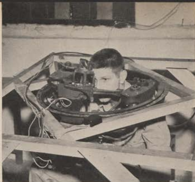
Mock-up of B-29 upper turret sighting station at overseas ground school of the 20th Air Force enables gunner to sharpen his eye.
