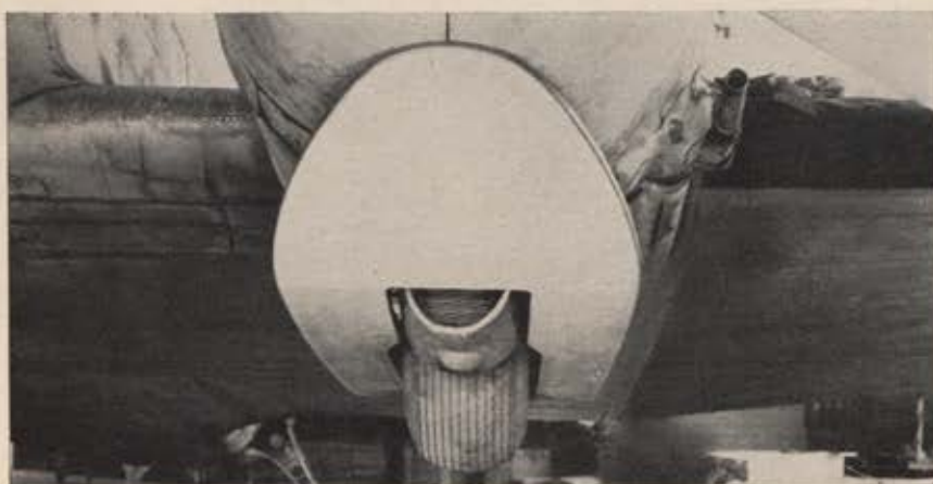
With skis mounted on its landing gear (shown retracted) a C-47 can land in snow.
