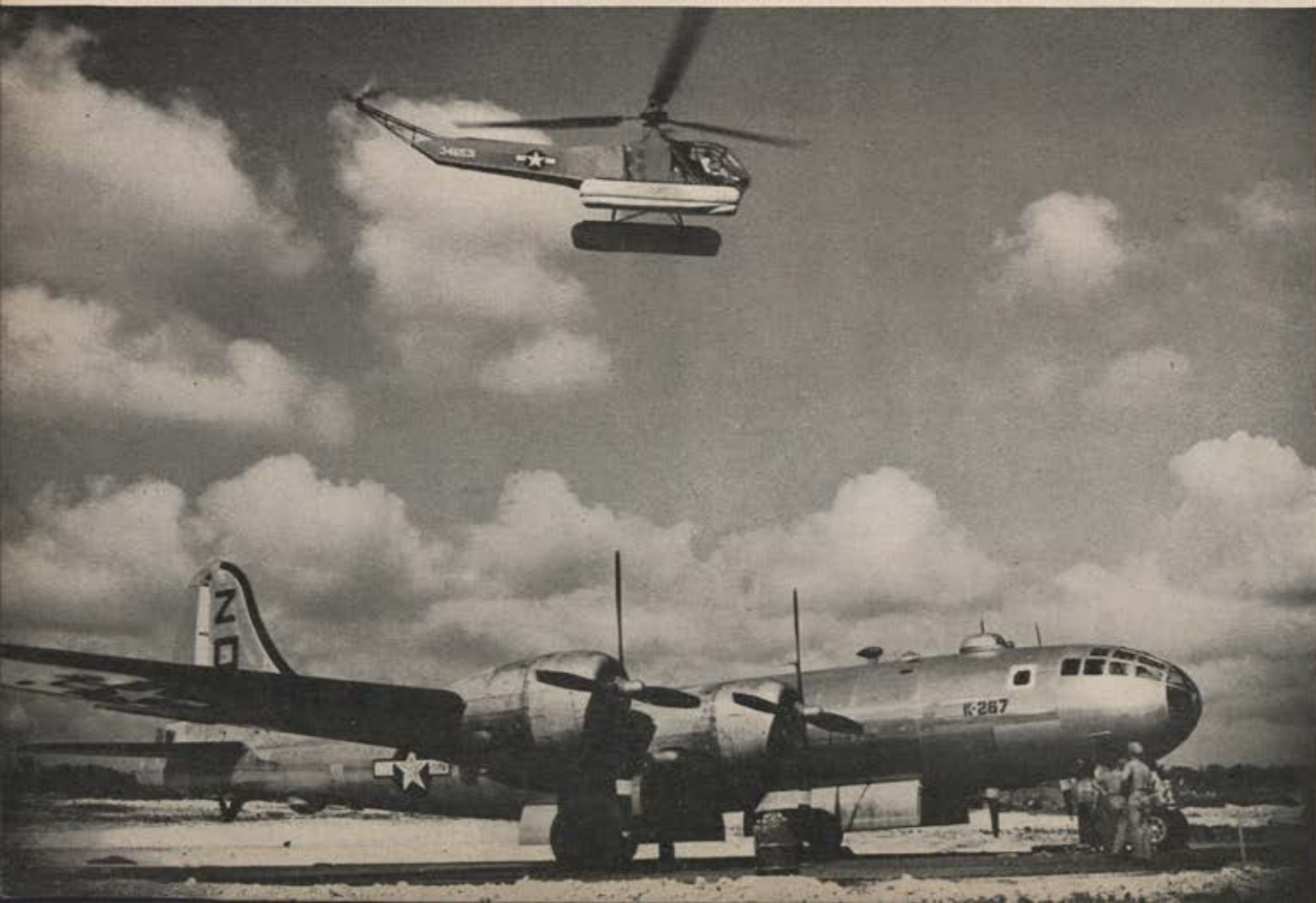
Personnel, tools, and spare parts are flown from the Liberty ships to B-29 airfields by R-4B helicopter to speed maintenance and repairs.
