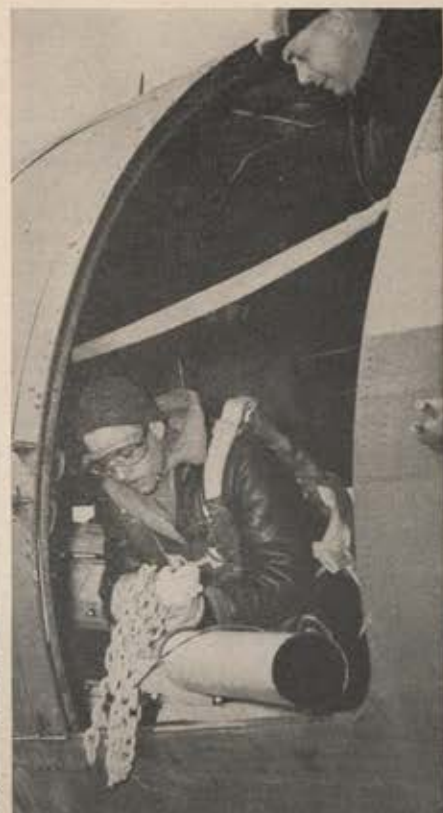
Telephone line laid by air over rugged terrain speeds communication between advance units and headquarters in ground fighting. At right, man prepares to drop plummet chain which will start wire through cargo door guide tube at the rate of 220 feet per second.
