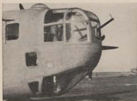
Modification to lead B-24s in Italy gives navigator front seat. Interior view (below) shows work table and space for instruments.
