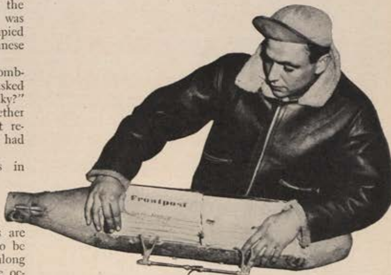
The German-language tabloid Frontpost , designed to give Germans the world news from an unbiased viewpoint, is distributed daily to enemy foxholes. It is carried in revamped practice bombs which open up on trigger release and dump the papers on their targets.
