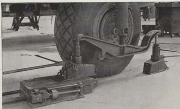
In the foreground is the scale unit with screw-type counterpoise on a weight-beam, which enables registering of weight up to 60,000 pounds. Beam is used primarily on dual-wheel landing gear (B-29 and C-54, for example) where space limitation does not permit jacking directly.
