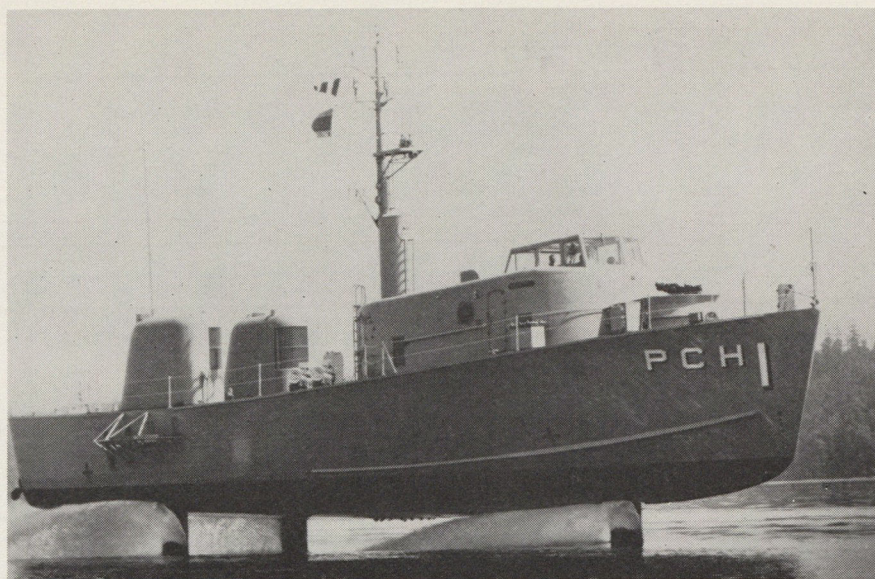
This is Boeing Company's hydrofoil vessel HIGH POINT, built for U.S. Navy to explore military potential in antisubmarine warfare. Powerplant consists of 2 Bristol Siddeley Proteus marine gas-turbine engines which can deliver "flying" speeds of 60 knots.
