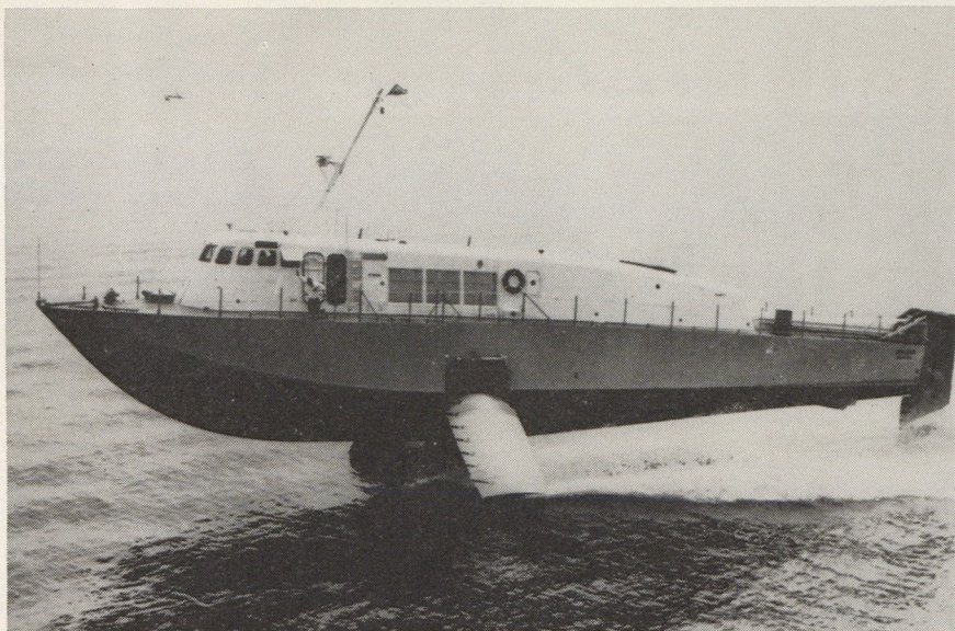
Grumman's hydrofoil ship DENISON, built for U.S. Maritime Administration, uses 2 surface-piercing foils and 1 submerged foil. The primary powerplant is GE LM 1500 marine gas turbine. In hull-borne mode, it is powered by 2 GE T58 gas-turbine engines.
