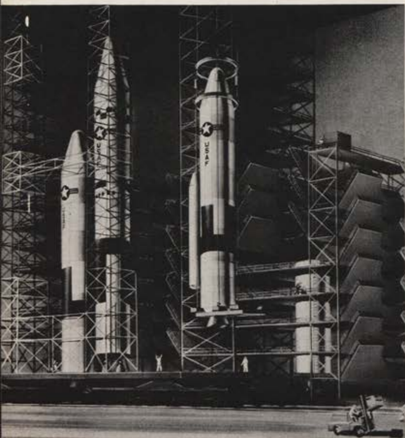
Large wind-tunnel model of the Titan III-C is readied for testing in transonic tunnel at Cornell Aeronautical Laboratory (below). Assembly and checkout of Titan III booster will take place in a building 215 feet high at Cape Canaveral (sketch above). Little checkout will be needed on the pad.
