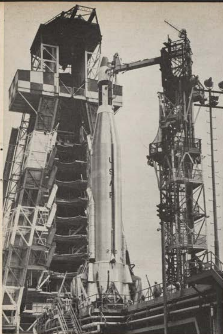
Close-up view of gantry tower used to prepare Atlas-Agena A for launch with Midas 2 payload. Platforms permit technicians to work on various parts of booster simultaneously. Midas 2 was successfully orbited in May 1960. These military satellites are now classified by DoD.
