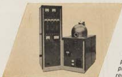
Unique semi-automatic equipment developed by LSi for mass production of integrated thin film microcircuitry.
