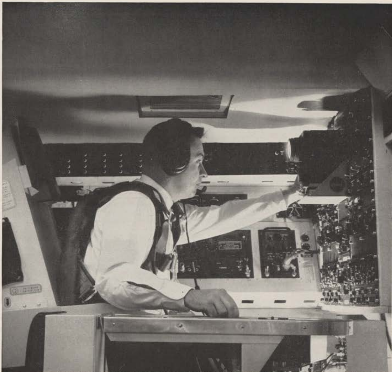
AN/ALQ-T4 IS THE FIRST COMPLETE ECM SIMULATOR DELIVERED TO USAF. PURPOSE IS TO TRAIN B-52 ELECTRONIC WARFARE OFFICERS.
