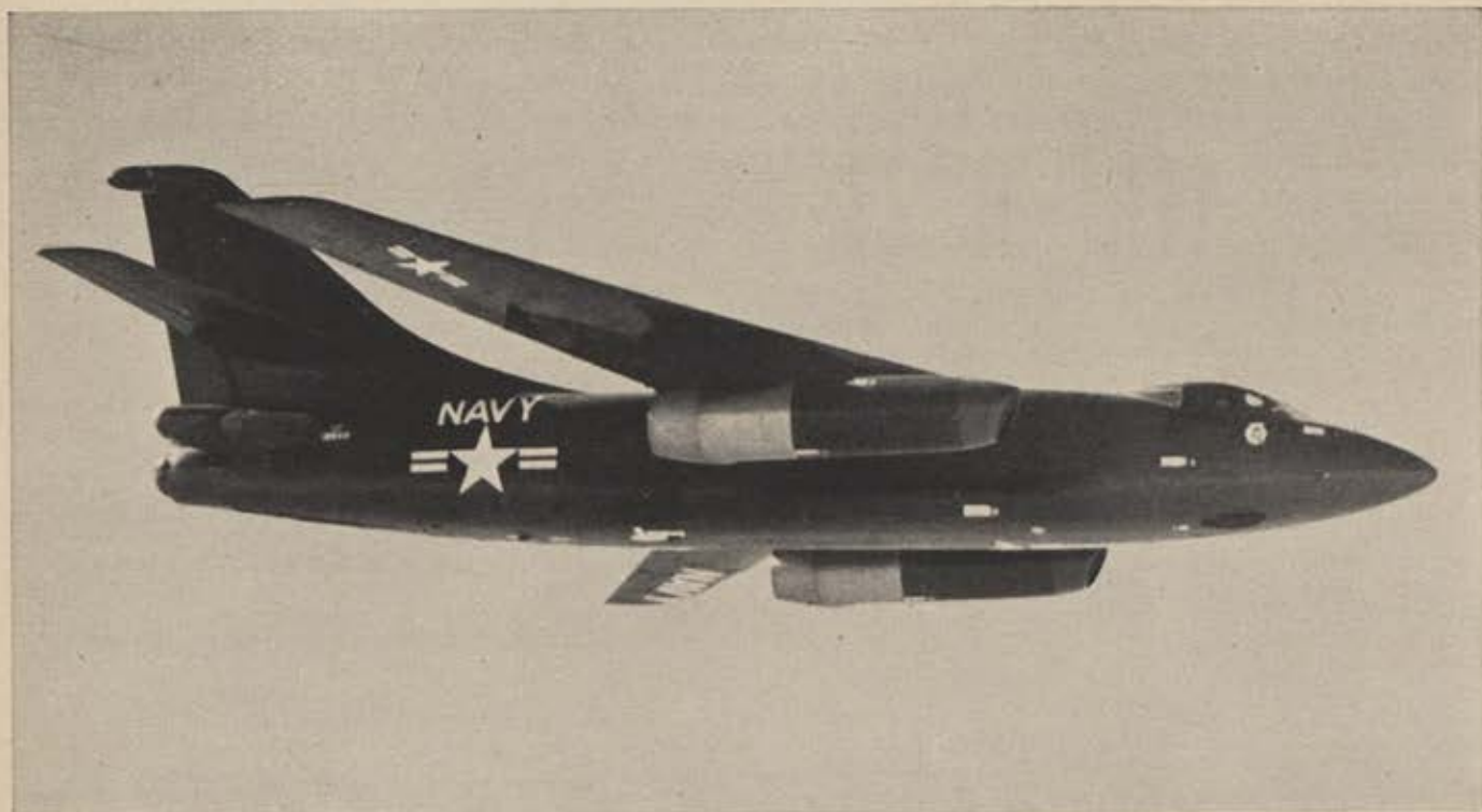
The new far-flying Douglas A3D, powered by two Pratt & Whitney Aircraft J-57 turbojets, is designed to be the Navy's most potent carrier-based aircraft—a major addition to U. S. Air Power. It is in the 600-to-700 mile-per-hour class.
