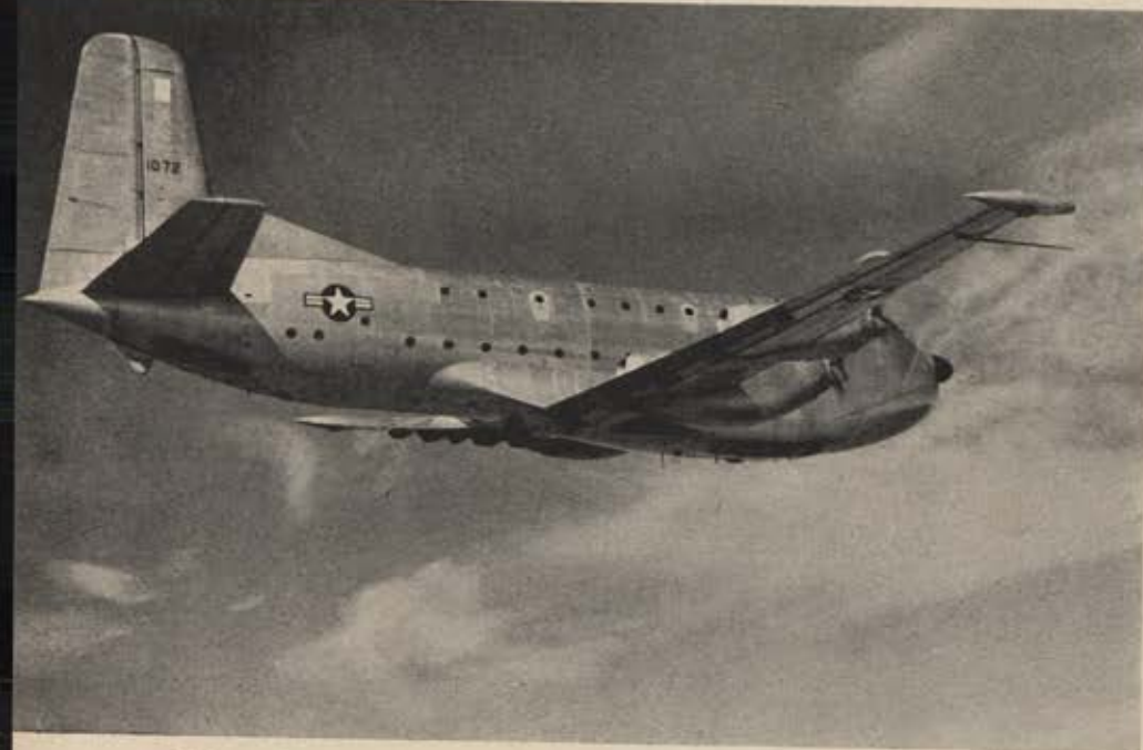
The turboprop-powered Douglas YC-124B is expected to cruise above 300 mph.
