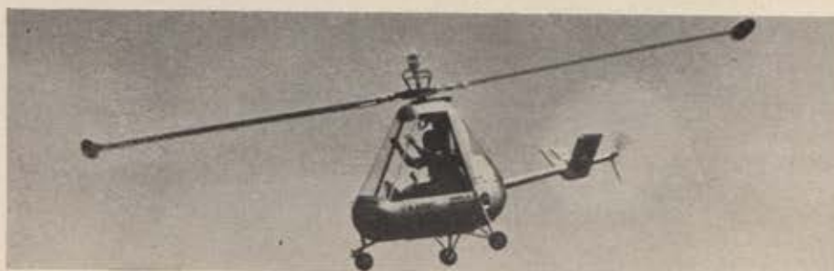
XH-26—One-man, collapsible, jet helicopter
