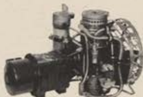
Airborne. 28v — 2 hp motor. Vertical sump. At sea level, and at 15,000 ft. delivers 2 cfm of free air compressed to 3,000 psi.
