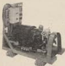
Ground application. Here a portable gasoline motor is used as a driving unit.
