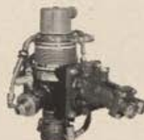
Airborne. Hydraulic drive. 3,000 lb. hydraulic system. Pressurized inlet. Remote sump.
