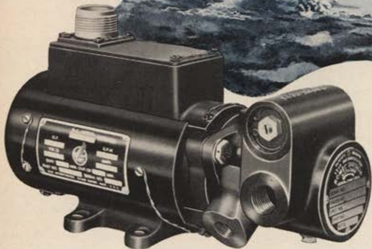
RG-9540 HEATER FUEL PUMP —6/100 hp electric motor driven, weight less than 4 lbs., rated capacity 35 gph at 25 psi discharge. Several hundred of these pumps have been manufactured for Boeing.
