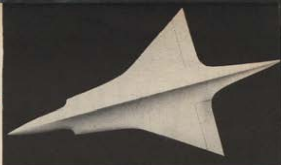
A model of the supersonic, blended hull configuration has a delta wing.
