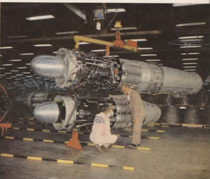
THRUST or "push" of G-E jet is increased by afterburner, shown on the top engine. Pilot can climb faster, gets greater bursts of speed in combat.
