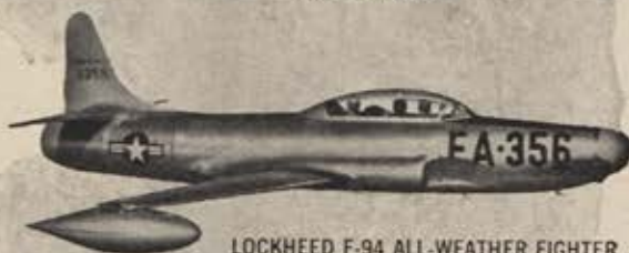
LOCKHEED F-94 ALL-WEATHER FIGHTER POWERED BY ALLISON J33 TURBO-JET WITH AFTERBURNER
