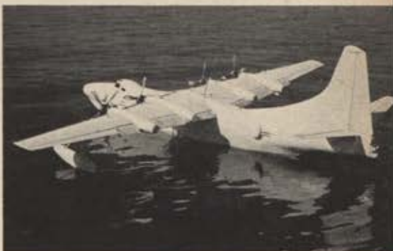
Flying model of XP5Y-1 was used to test hydrodynamic characteristics.
