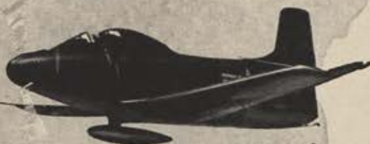
DOUGLAS A2D SKYSHARK POWERED BY ALLISON T40 TURBO-PROP
