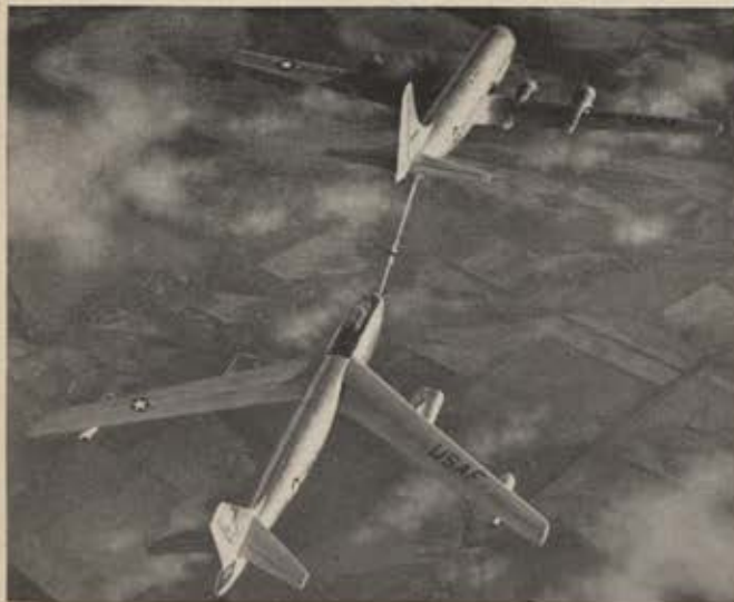
The C-97, as tanker, refuels the B-47; also jet fighters.
