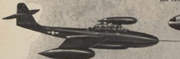
NORTHROP F-89 SCORPION POWERED BY TWO ALLISON J35 TURBO-JETS WITH AFTERBURNERS
