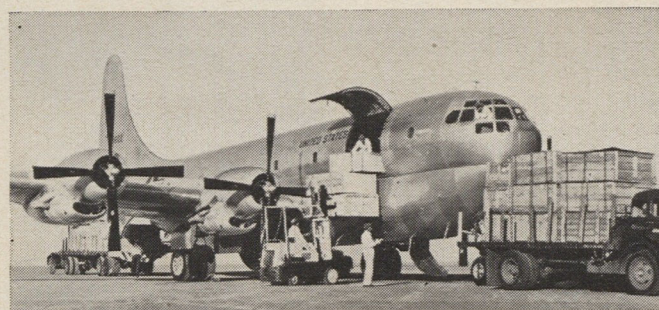
...and a heavy cargo carrier! Stratofreighter can be loaded with 34 tons of freight from four trucks simultaneously.
