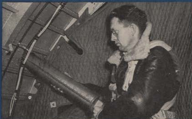
Temperature of the outside air is taken by an engineer inside a C-53. It is done by sticking poles wrapped in sensitive paper out into windstream.
