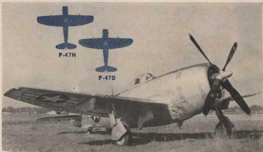
Squared-off wing tips, greater span and added aileron area give P-47N superiority over P-47D.
