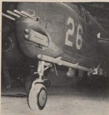
Nose on latest model B-25 bristles with increased armament. Four machine guns are mounted above three fixed rocket launchers.
