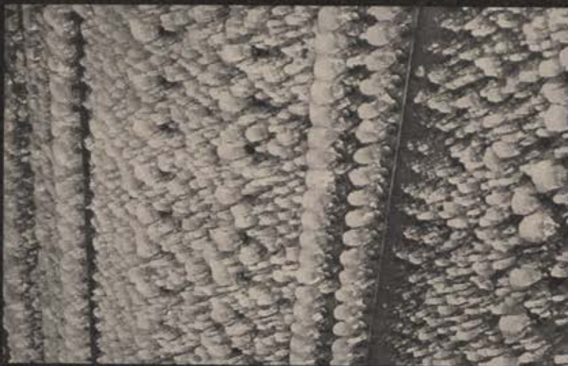
Rime ice has formed on the lower forward section of this wing. It is made up of white, rough crystals which build up and grow out to the windward.
