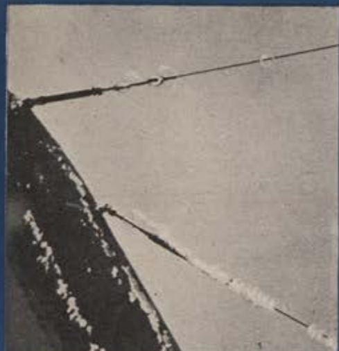
Action of a deicer boot along the leading edge of the vertical fin kept this section cleared.
