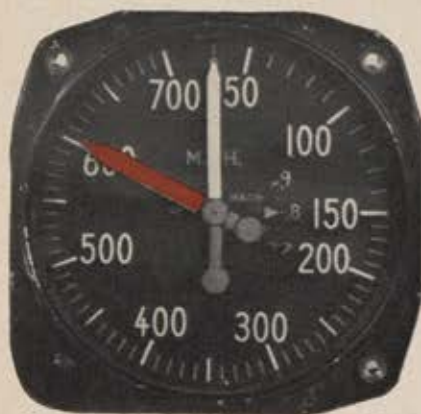
In new type airspeed indicator, red dial varies with altitude to give warning when the plane is approaching a critical speed.
