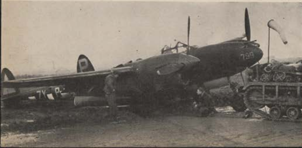
Belgium. Slippery landing strip caused this Lightning to skid off runway. Mud forms when drainage ditches can't handle constant rain loads. Rapid wear of brake drums and linings, broken axles, stripped gears are among mud's victims. Rocks stuck in mud damage tires.
