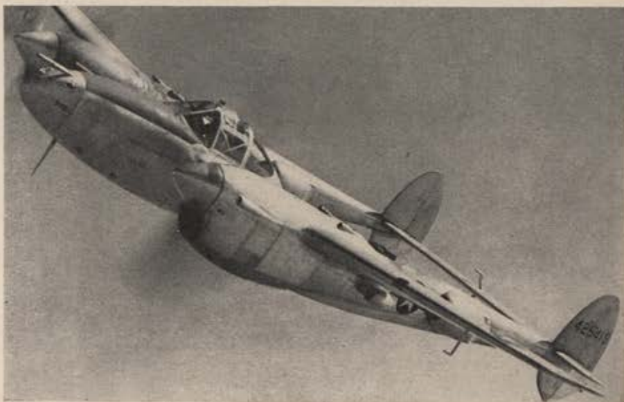
P-38L features compressibility flaps, new supercharger devices and a cockpit heating system.
