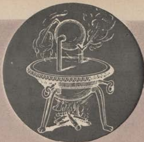
One of the earliest demonstrations of jet principle was Hero's aeolipile, which converted steam pressure into mechanical force in days of Alexandrian culture.
