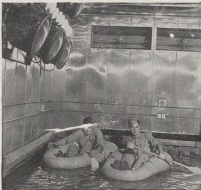
Blizzards rage and storm winds blow in the all-weather chamber of the Aero-Medical Laboratory at Materiel Command headquarters. Testing life rafts is one of many uses made of this storm center at Wright Field.
