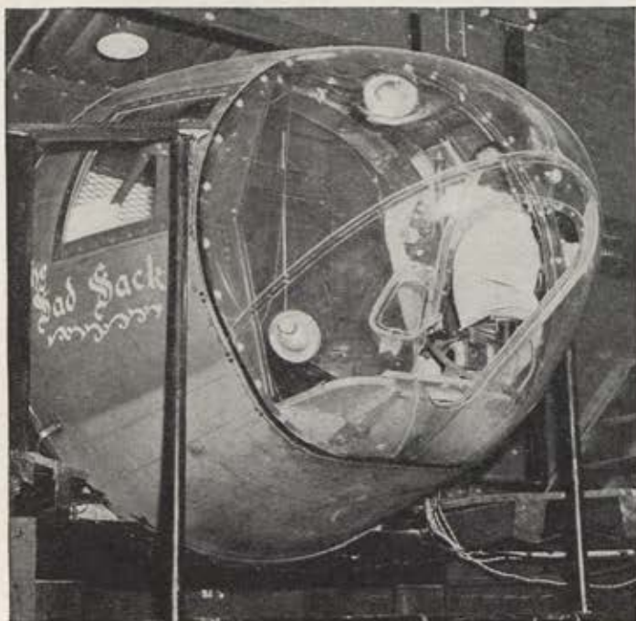
The bombardier soon learns the difference between a bombardier and a combat bombardier. While making his "runs" in this bomb trainer, an electrically operated device which provides air speed and drift problems, the bombardier is subjected to aircraft sounds, gunfire and simulated flak puffs.
