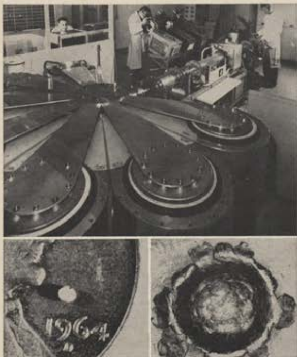
This electrothermal gun device fires synthetic micro-meteoroids at speeds up to 12 mps at North American Aviation Lab, Downey, Calif. Lower left, micrometeoroid (white sphere) shown on head of penny. At right, a closeup of crater caused by the projectile.
