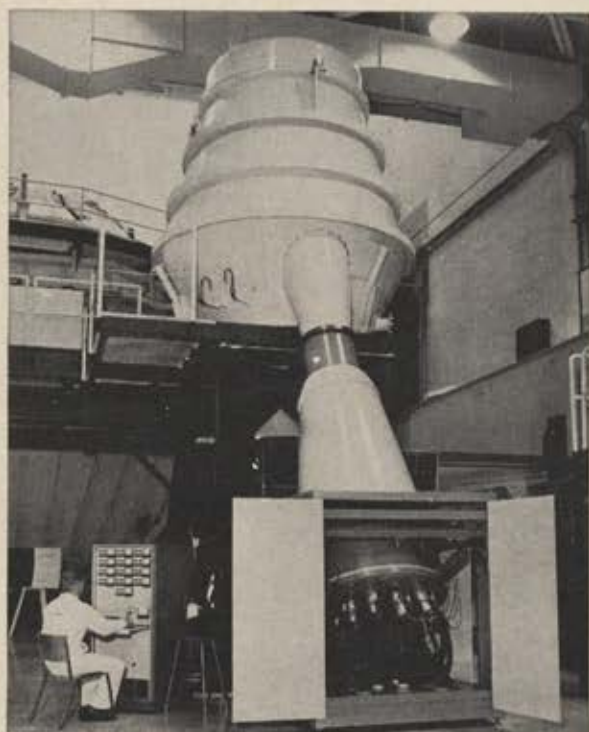
This solar simulator at Douglas' Space Systems Center, Huntington Beach, Calif., generates a four-foot-wide, 270-watts-per-square-foot intensity, enough to simulate Venus solar environment. Used in vacuum chamber, it will test spacecraft response to sun's heat.
