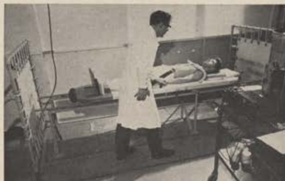
Boeing space-medicine researchers are studying potential of bed-trampoline device to aid conditioning in zero-gravity. Volunteer lies motionless on sliding bed while being subjected to 1.5 Gs at each bounce. Intermittent G-loads "exercise" the cardiovascular system.
