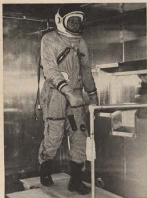
Body-moisture buildup can be a hazard to cold-weather survival. At Division's Protective Equipment Section, Ft. Wainwright, Alaska, a subject does mild walking exercise at 30 degrees below zero to check actual amount of buildup in subzero condition.
