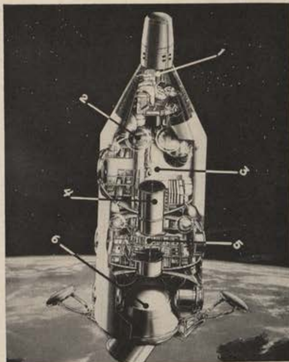
Artist's conception of Lockheed's proposed MOL configuration. Features include (1) Gemini capsule for astronaut transit, (2) spheres for fuel and equipment storage, (3) living compartment, (4) air lock between compartments, (5) lab compartment, and (6) camera.
