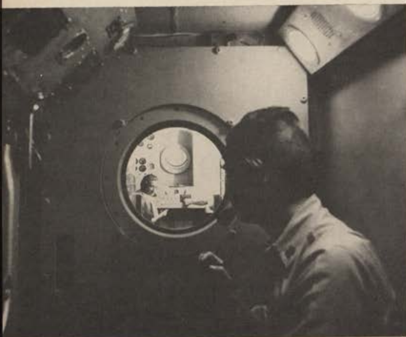
In place at USAF's School of Aerospace Medicine at Brooks AFB, Tex., is the versatile manned space simulator chamber. The simulator provides capability for a wide range of atmospheric mixes within an area comparable to that of the projected Air Force Manned Orbiting Laboratory two-man space capsule.
