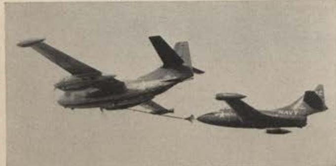
FR package equipment, quickly mounted in bomb bay, turns bombers into tankers, gives carrier-based fighters far greater range.
