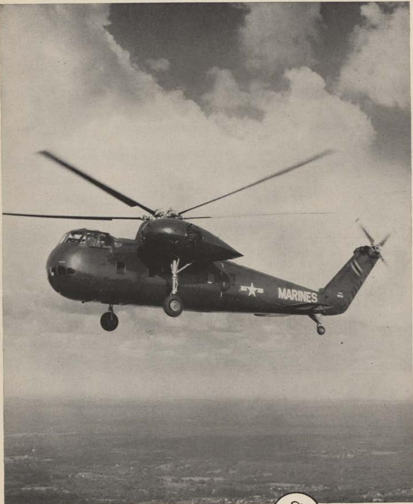
**BUILT FOR BATTLE**—Sikorsky Aircraft's rugged XHR2S, the most powerful helicopter now flying, was designed to carry out modern vertical assault tactics. It has flown with over 6,500 pounds of payload, and at speeds well over 150 m.p.h. with landing gear retracted into engine pods. Five-bladed main rotor and the tail both fold mechanically for easy stowage and handling aboard ship.
