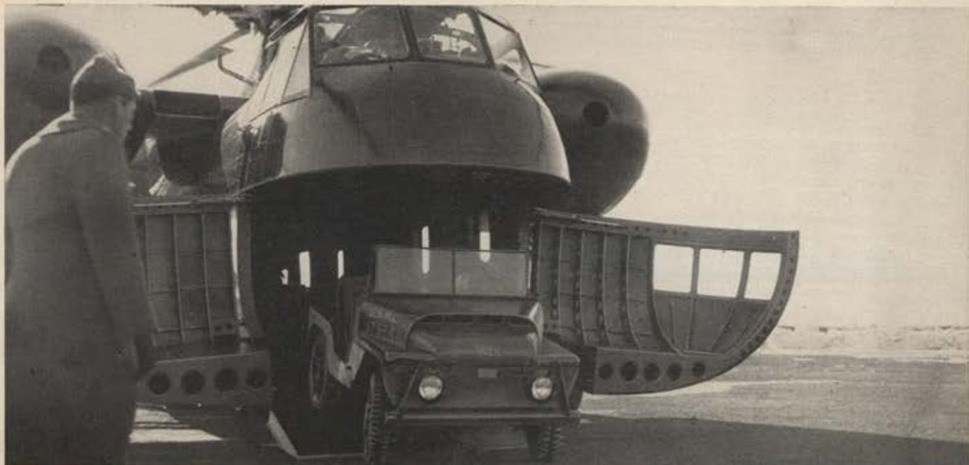
**PRACTICAL DESIGN**—Location of two R-2800 engines in high, outboard pods leaves the fuselage open and clear for passengers, vehicles or other cargo. Wide clam-
