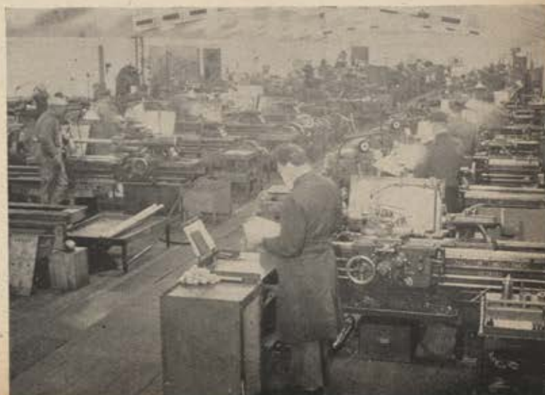
Above, one of the underground workshops. The factories are lighted by a combination of mercury vapor and incandescent lamps. Air conditioning keeps the temperature comfortable no matter what the weather outside. Below, another inside view of the workshop.
