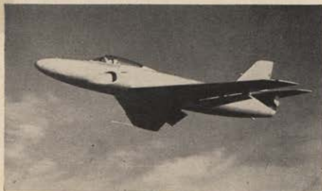
The Lance, a two-seater, all-weather jet, goes into mass production in about a year. A Rolls-Royce Avon powers it.
