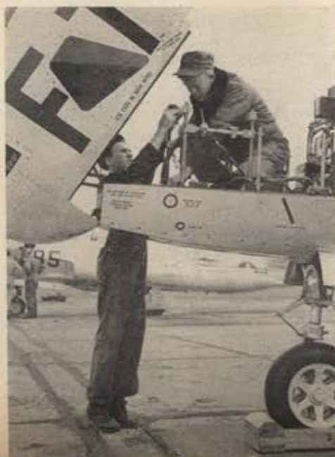
Guardsmen on active duty install a camera mount in the nose of an RF-80, one of the planes belonging to the 117th Tactical Recon Wing, the first USAF recon outfit to be assigned to Europe.
