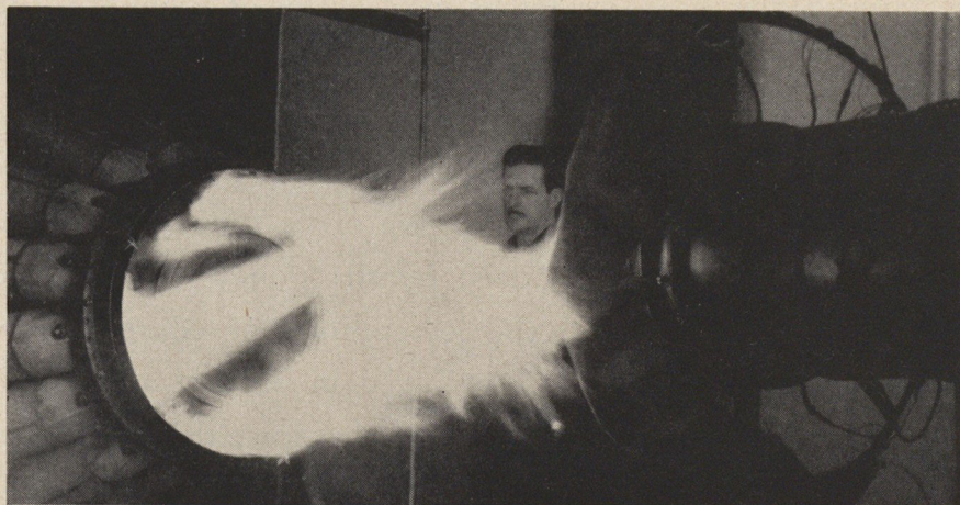
Above, starting test of a J-33 jet engine with tail cone removed to study flame propagation of ignition. Below, the tops of forty-foot distillation columns in which precious aviation experimental fuel compounds are purified.
