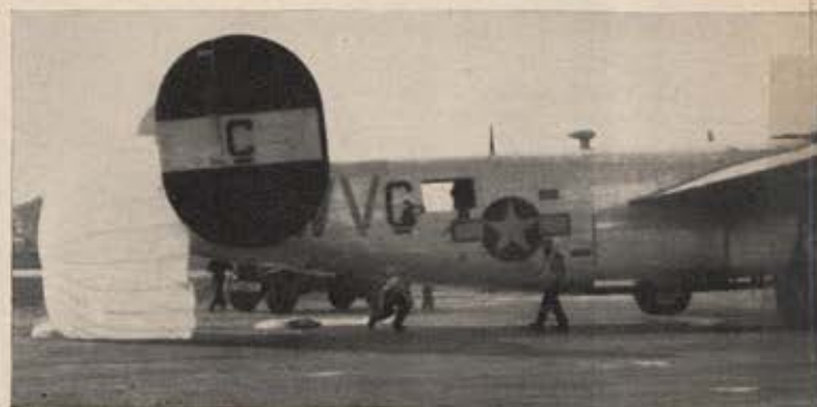
GI ingenuity saves the day for a B-24 whose hydraulic system was shot out over Germany. Parachutes released through the waist windows of the brakeless Liberator, just before the wheels touched, effectively slowed it down.
