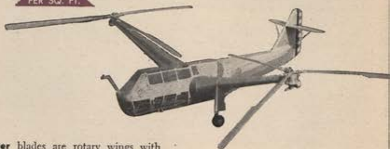
Helicopter blades are rotary wings with changeable pitch to give thrust and lift.
