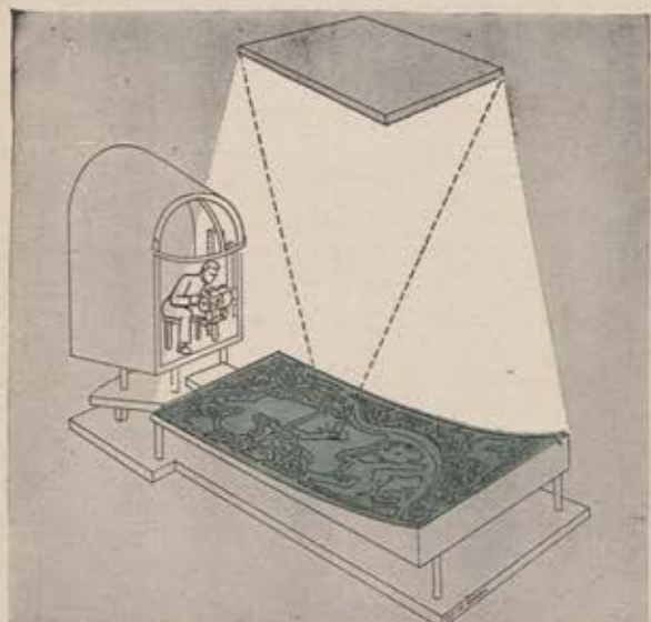
Film of moving terrain is projected onto overhead mirror where image is reflected back to screen below, duplicating bombardier's view. Trainee sits in fully equipped mock-up of bombing station, ready to "release" his simulated load.
