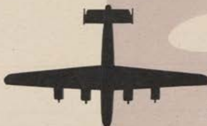
B-24 uses Davis wing with a reverse curve at trailing edge.
