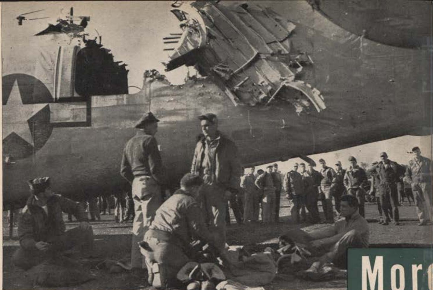
This B-24 blew its top when flak burst in waist section during mission over Yugoslavia. The shell blew out both guns, severed the rudder control cables, killed one gunner. Pilot guided the Lib home using only the engines.
