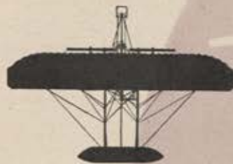
Wing of Wright Bros. 1908 model had wire trailing edge.
