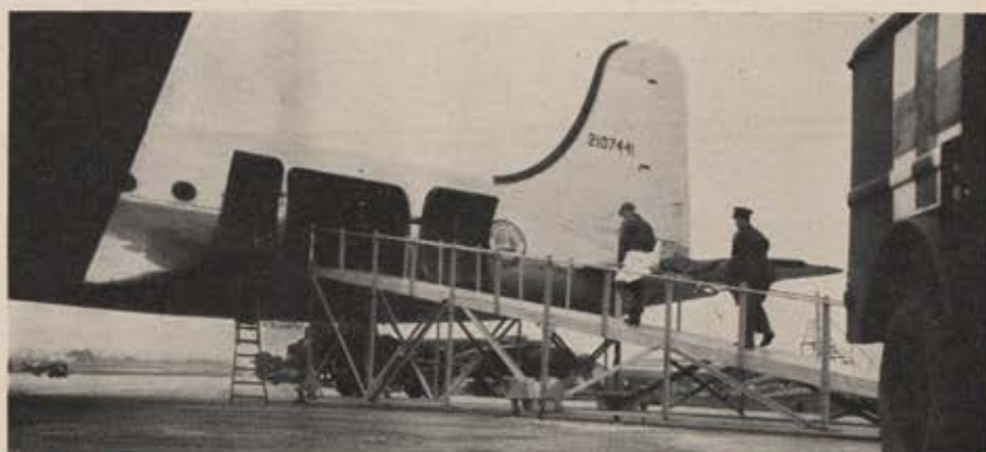
At the ATC's European Division terminal in Scotland, a wounded American is carried aboard a C-54 by way of home-designed steel ramp. In two parts, bottom section alone loads C-47s.
