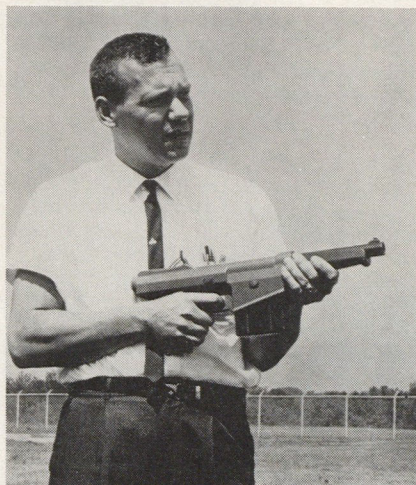
This is the latest in a family of Avroc weapons being developed by Avco Corporation. The 20-pound (9 kg) Avroc 5-20 fires 5-mm. projectiles by means of a rocket motor, which eliminates need for cartridge. Exhaust gas recycles the gun.
