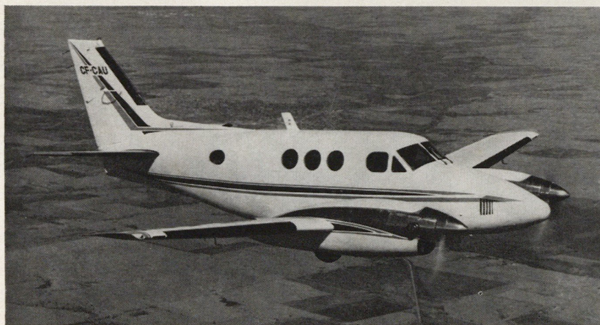
A new airborne system, UNACE (Universal Aircraft Communication/Navigation Evaluation), installed on Beech Aircraft Corporation's King Air, was purchased for calibration purposes in December by the Canadian Department of Transport. UNACE, designed to simplify inspection from the air, can check all airway electronic and radar installations.
