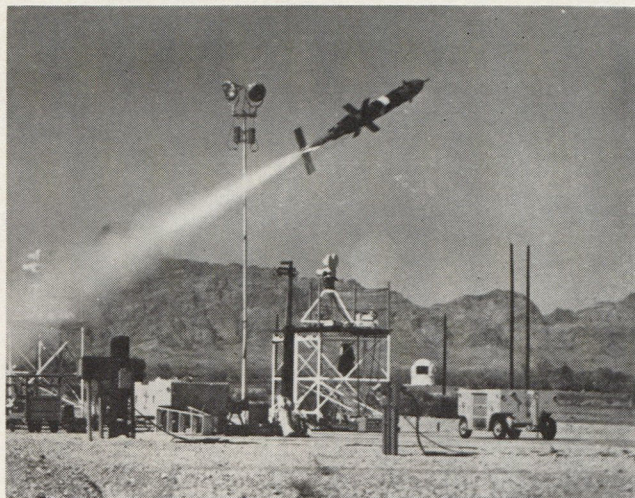
The CL-89, now designated the AN/USD-501, is launched by booster rocket and has a turbojet sustainer engine. Carrying sensor equipment, it provides tactical information for Army formations in battle areas. It is recovered by parachute and reused.
