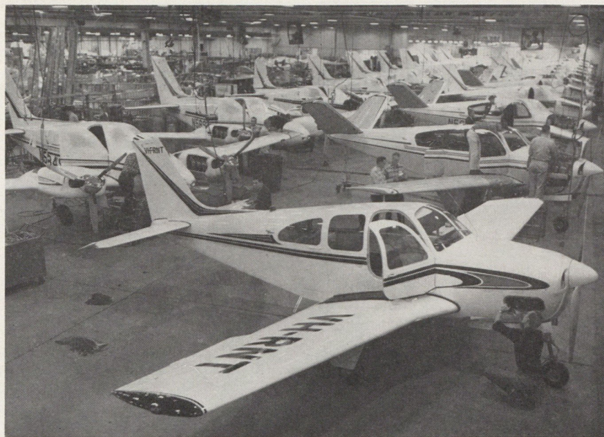
This is the Beech assembly line at Wichita, Kansas, one of the manufacturing sites of the famed general-aviation firm. The company is one of the industry's leaders, and its aircraft fly the American general-aviation airlines, carrying businessmen about the U.S.
