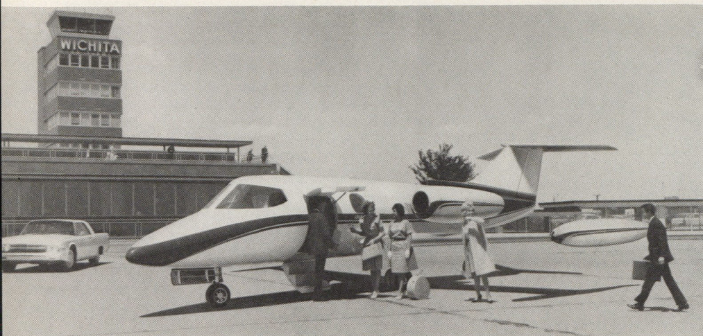
The Lear Jet Model 23 has gone a long way toward proving that there is a large market for the 5- to 9-passenger business jet. The Lear Jet is the smallest in the field, carrying 5 or 7 people. It is derived from a fighter design and is an outstanding performer from an aeronautical point of view, with a roomy and luxurious interior style.
