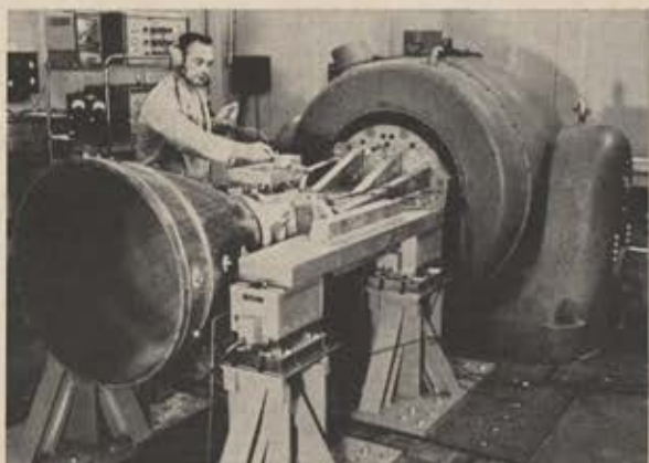
NASA's Lunar Excursion Module ascent engine gets shakes at Textron's Bell Aerosystems, Buffalo, N. Y., facility on a new vibrator, produced by MB Electronics, New Haven, Conn. The vibrator produces 28,000-pound force, frequencies up to 2,000 cycles per second.
