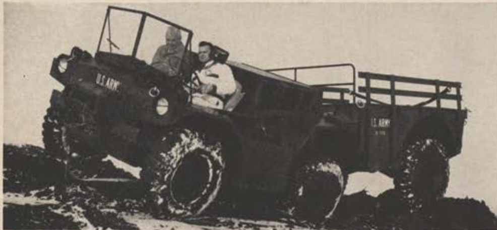
PATA crosses hard and soft terrain on continuous track of air-filled cells.
