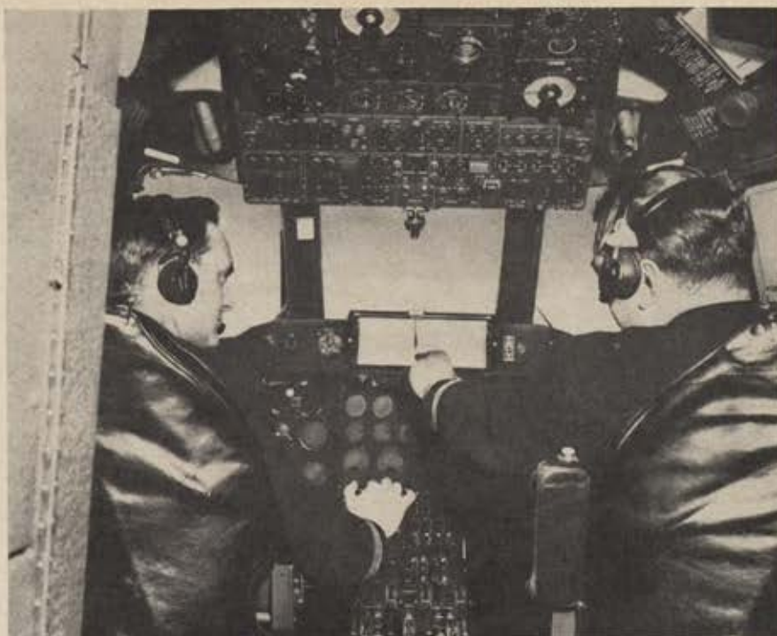
The Decca Flight Log indicator continuously presents current position and past track of the aircraft ... the ultimate in pictorial presentation.
