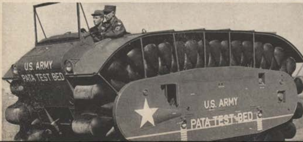
PATA crosses hard and soft terrain on continuous track of air-filled cells.
