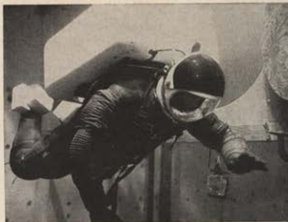
Boeing's zero-gravity researchers have reported progress in their studies using a submerged, water-filled facility in which weightlessness is simulated. In zero-g-like environment, researchers are able to study personal locomotion and equipment handling.
