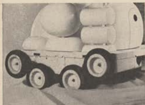
Vehicle can shorten wheelbase for tight maneuvering. If necessary, it can lock wheels and rotate beams to literally "walk" through soft ground.
