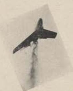
The sleek new fighter taking-off on this month's cover is the Republic F-84F Thunderstreak, swept-wing version of the Thunderjet, one of the work-horses of the Korean air war. But the F can fly higher, faster, and farther, and packs a bigger wallop. Chuck Barnes made the drawing from a color photo. For more about the F-84F, see page 29.
