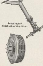
Segmented Rotor Brakes
