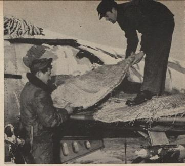
During protracted periods of snowy weather, the guys on the ground in Korea cover the wings of their ships with rice bags, above. Then, if the weather breaks, even for a few moments, they will be able to get their planes off the ground into action.
