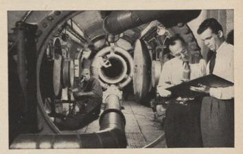
Full scale compressor test stand in new Aircraft Gas Turbine Laboratory at Lynn, Mass. can run tests simulating altitudes up to 70,000 feet, temperatures to ±100F. The lab, newly opened, is dedicated to memory of Dr. Sanford Moss, early pioneer in aviation.
