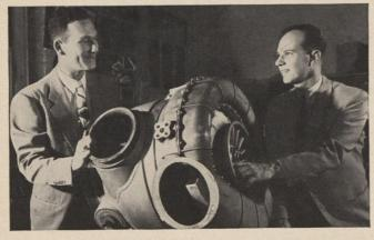
New turbosupercharger promises longer ranges, heavier payloads to today's transport aircraft through greater power, lower fuel consumption, and greater simplicity. Now on test with Pratt and Whitney R-4360-C engine, it can be adapted to any engine of similar size.
