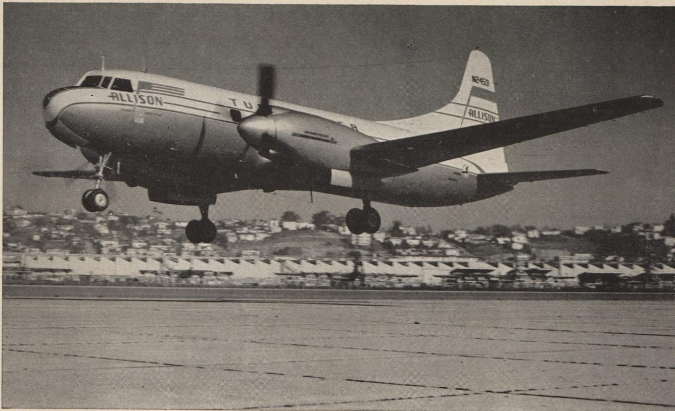
The Convair Turboliner, powered by two Allison 2750 hp. turboprop engines, makes its initial takeoff from San Diego field.
