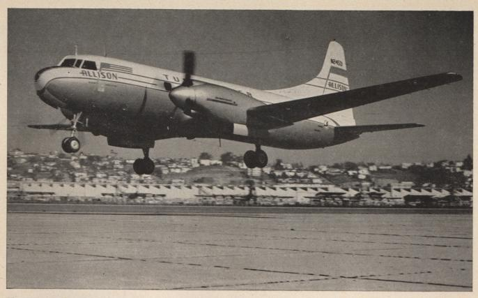
The Convair Turboliner, powered by two Allison 2750 hp. turb oprop engines, makes its initial takeoff from San Diego field.
