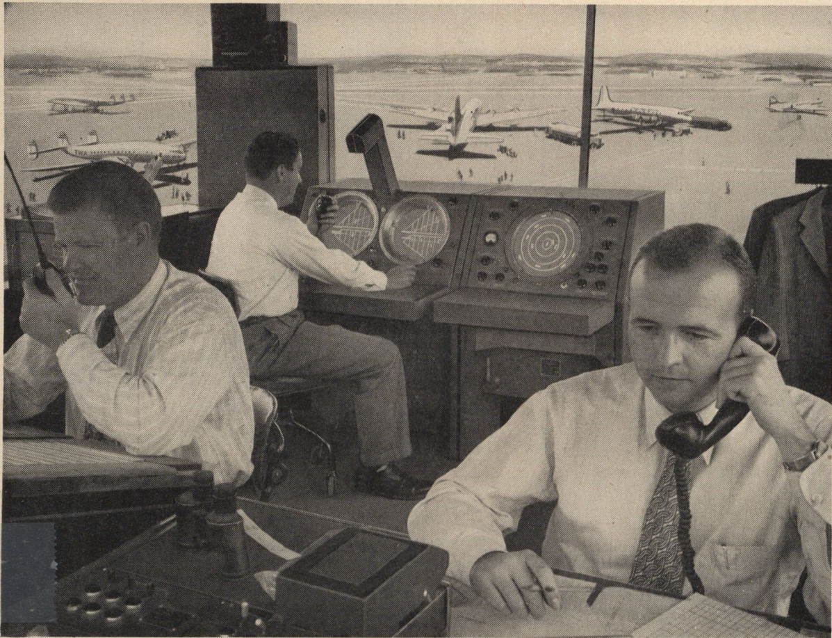
GILFILLAN'S GCA CONSOLE in the L.A. control tower contains a surveillance scope (right), and two precision scopes for blind landings. On the left is the three-mile final approach scope; in the center the 10-mile scope. Aircraft's position on final approach is shown in three dimensions accurate to \pm 15 feet.
