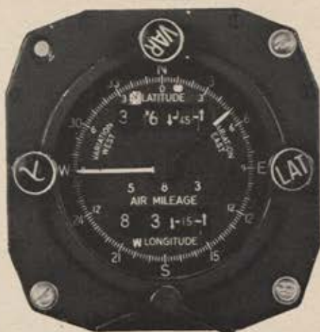
Instrument computes factors in diagram below and indicates air position on face of dial.
