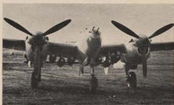
Here are P-38s ready to go on the war path. P-38 in top photo carries belly tank and 1,000 lb. bomb. These planes hit refinery shown at left. Bottom P-38 packs six 500-pounders, used for high-level or dive-bombing.
