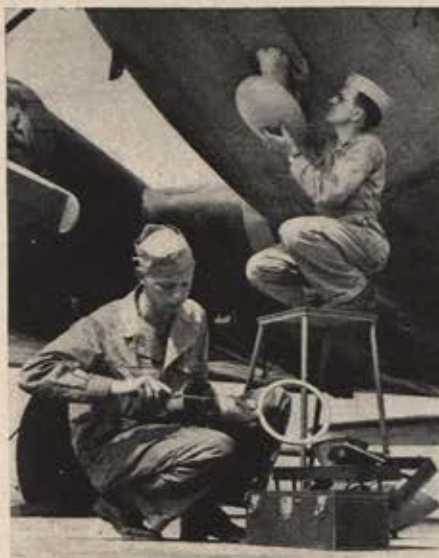
Radio mechs change loop antenna to smaller size in streamlined housing. Antenna shown in foreground had created excessive drag.
