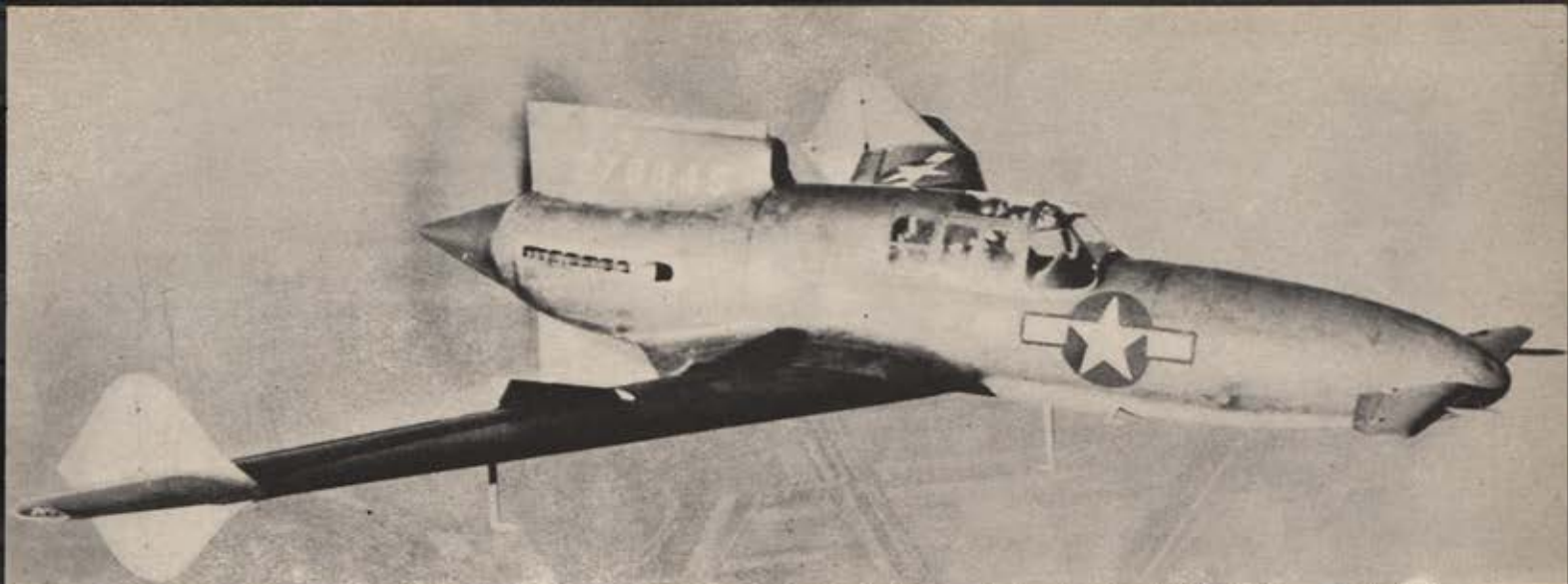
XP-55. Embodying some of the control principles of the flying wing, the Curtiss XP-55 has elevator controls in the extreme nose. Minus conventional rudder, the plane has vertical stabilizers near
