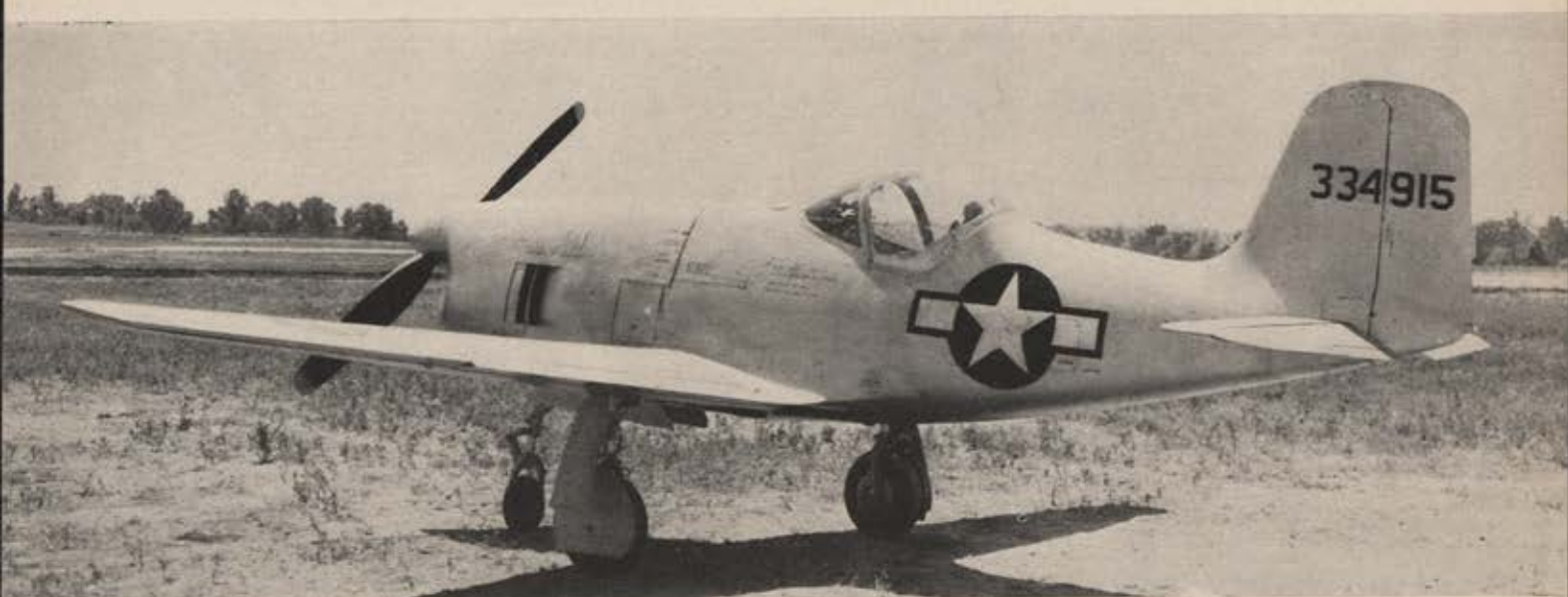
XP-77. Only all-wood AAF fighter of the war, the Bell XP-77 was built when metal shortage loomed critical. Hollow propeller shaft permits use of single forward-firing cannon. Powered with
