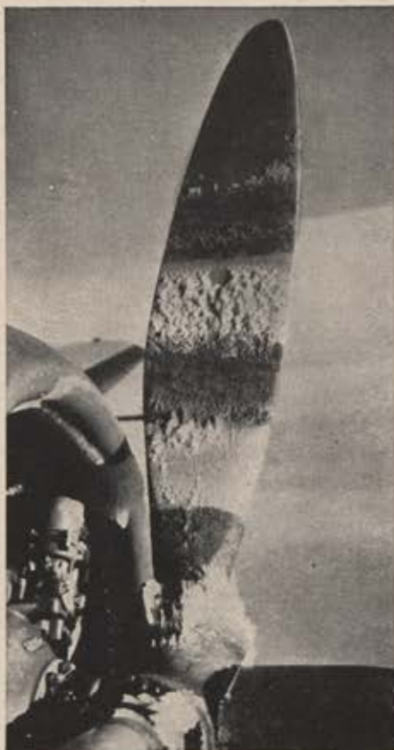
Ice formations on propellers pose a problem for ATSC engineers, who must eliminate such conditions without impairing prop efficiency.
