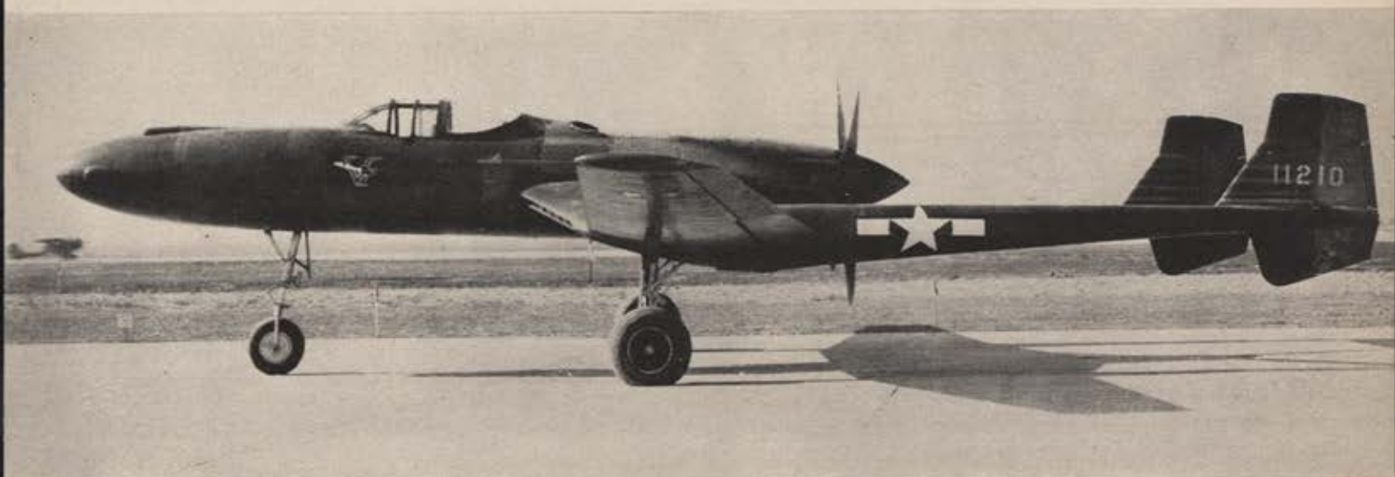
XP-54. First AAF pusher-type fighter since the twin-engined Bell XFM-1, Vultee's twin-boomed, bullet-shaped XP-54 introduced a low drag airfoil section, was one of the first planes to have flush-
