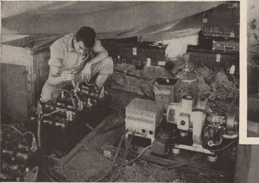
Airplane batteries are recharged in this "hangar." Extra care is necessary because spare parts are virtually nonexistent.
