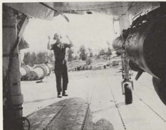
Heavily armed A-4 is directed out for takeoff at Chu Lai by Marine Pfc. Ray Markley. The aluminum matting forming the Chu Lai strip was laid on deep sand stabilized with asphalt.
