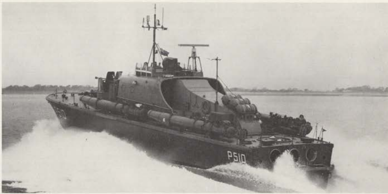
Danish Navy is acquiring a number of these fast patrol boats employing 3 Proteus turbine engines plus 2 small diesels, offering long cruise range with high-speed capability when needed. Denmark has also ordered a pair of frigates, which will be equipped with 2 Pratt & Whitney FT4 gas turbines for boost power in high-speed operations. FT4 is marine equivalent of engines in Boeing 707.
