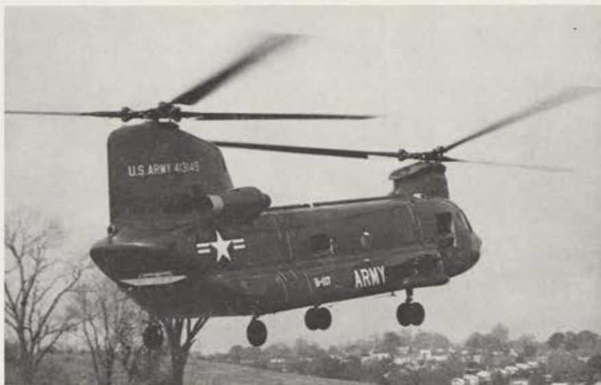
Displaying a variety of weapons, the first armed version of U.S. Army CH-47A Chinook helicopter was demonstrated for U.S. Department of Defense officials recently at Philadelphia International Airport, Pennsylvania. The Boeing Company's Vertol Division is currently assembling a number of Chinooks armed with M5 automatic grenade launchers, pylons equipped with 20-mm gun and rocket pod, and machine guns on side and rear.
