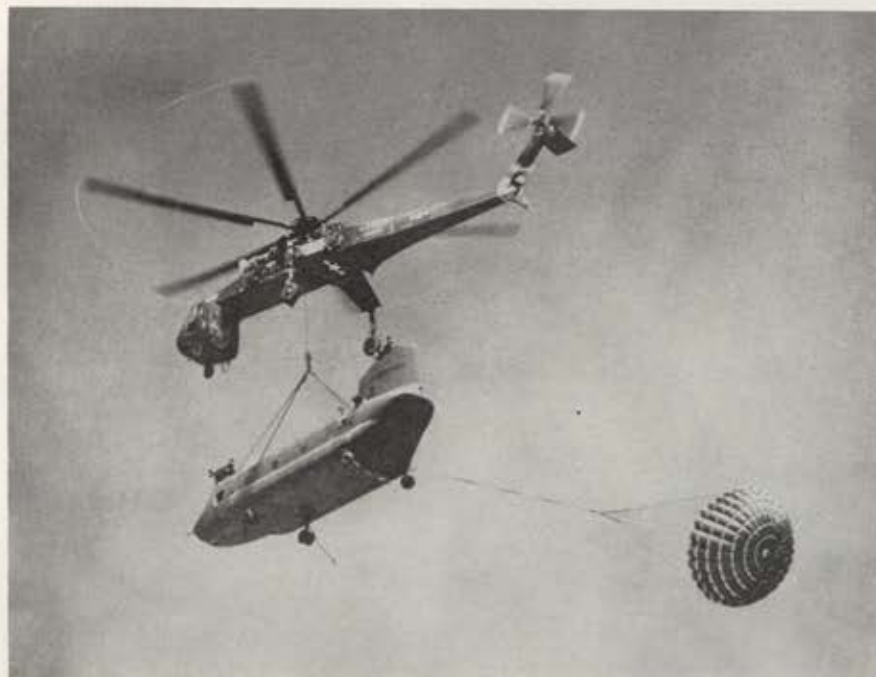
Demonstrating its recovery ability, Sikorsky CH-54A Skycrane rescues twin-engine Boeing-Vertol CH-47 Chinook helicopter that had suffered landing damage in Vietnam. Chinook airframe, weighing 14,000 pounds (6,350 kg), was carried on 4-point nylon sling, with drag chute stabilizing the load. Four Skycranes are flown by 478th Transportation Company with U.S. Army's First Cavalry (Airmobile) Division in Vietnam.
