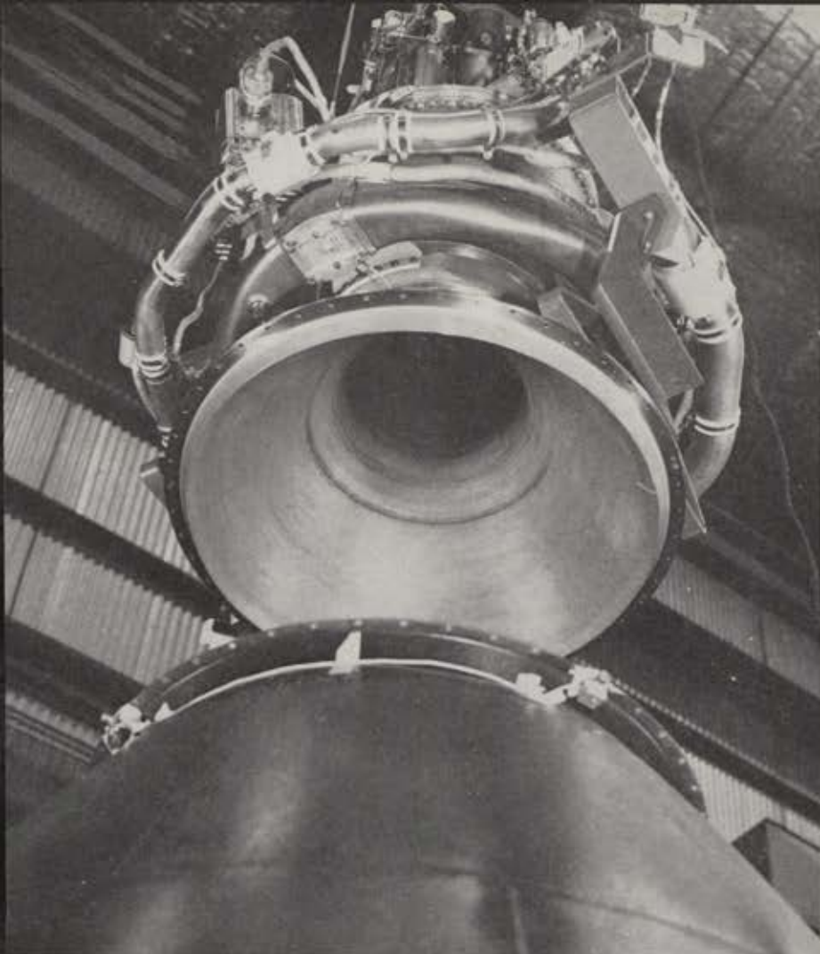
The Apollo service module propulsion system, which was test-fired recently at Cape Kennedy, Florida, is shown above being manufactured by Aerojet-General Corporation. It will provide power after booster separation for the trip to the moon and the return.
