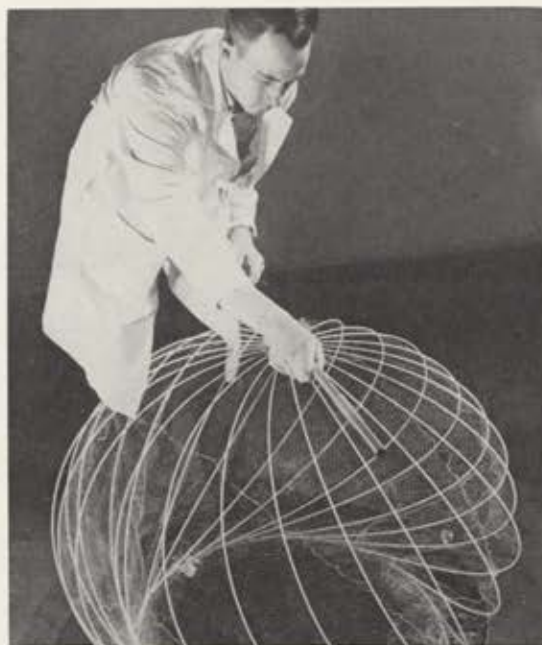
Lightweight antenna made of aluminum-coated nylon mesh supported by fiberglass rods is shown at left. It can be compressed into a briefcase-size package for launching into space, where it then will expand to a 60-foot (19 m) structure for reflecting high-frequency radio signals.
