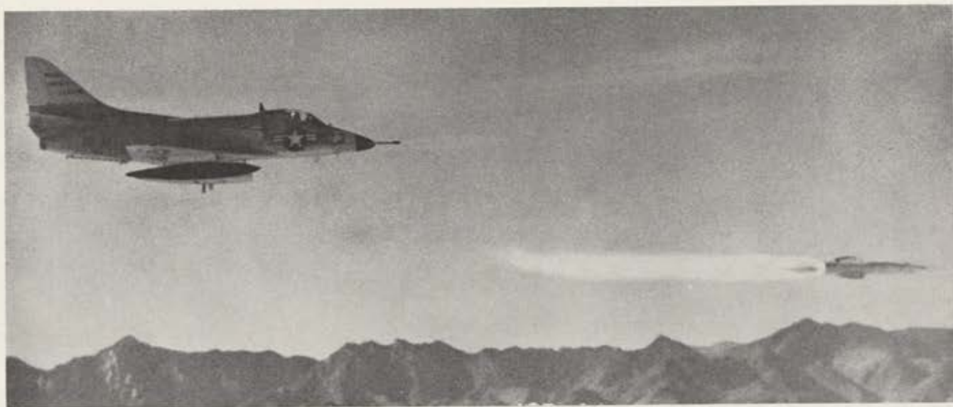
A wide variety of armament loads can be accommodated on the A-4. One of the most important weapons, the Martin-Maxson Bullpup, is shown being launched above. The Bullpup has been used in action many times in Vietnam by A-4 pilots, employing its radio guidance feature to destroy pinpoint targets such as radar antennas, antiaircraft emplacements, vehicles, and concrete command posts.
