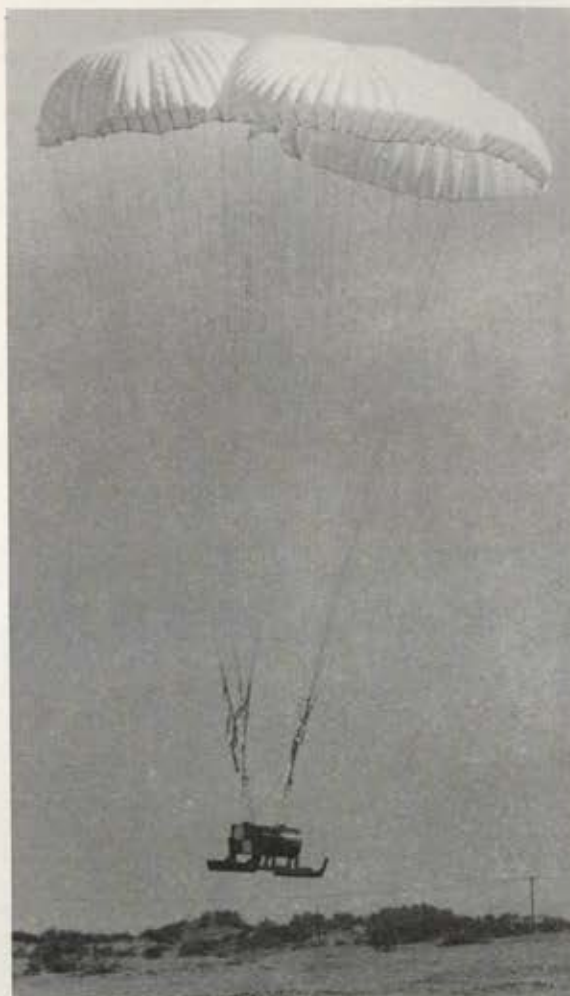
This 40-foot-diameter (12 m) model of the Northrop Corporation's Cloverleaf parachute descends with test sled in flight test of the controllable gliding chute at DoD Parachute Facility near El Centro, California. Under a new NASA contract, Northrop Ventura will develop a large Cloverleaf, test vehicle, and control system for pinpoint recovery of 5,000-pound (2,270 kg) vehicle leading toward precise landings of space vehicles.
