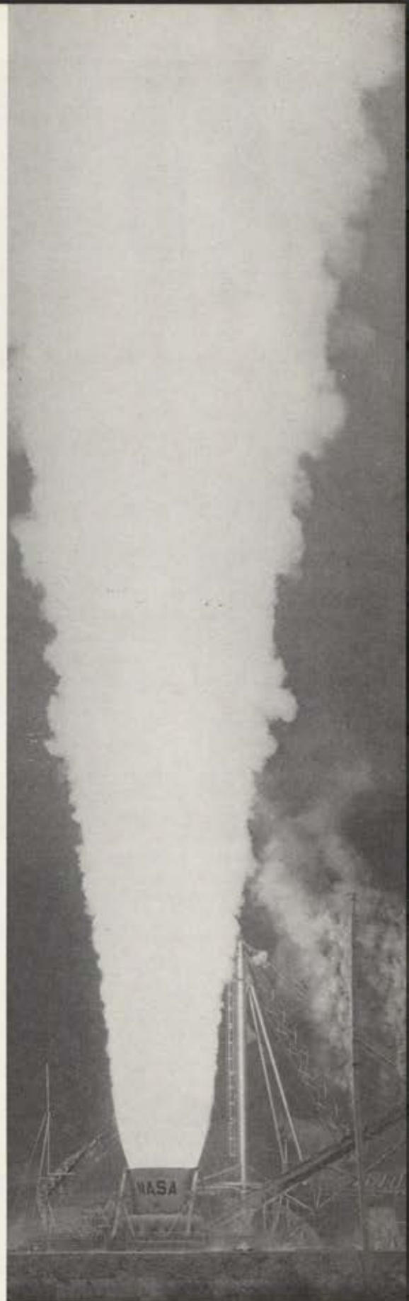
A plume of smoke several hundred feet high rises above the 260-inch diameter (660 cm) solid-propellant rocket recently tested successfully by Aerojet-General Corporation. The motor produced some 3,000,000 pounds (1,350,000 kg) of thrust.
