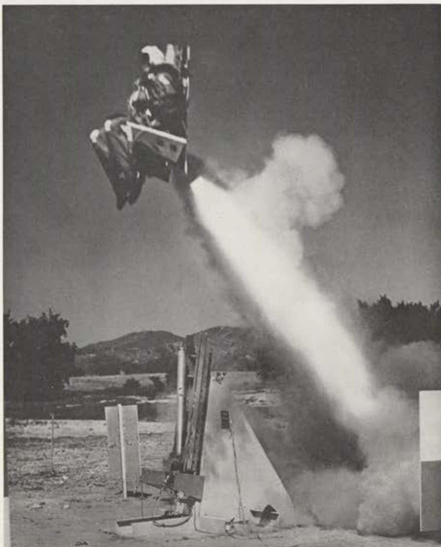
First live test of a zero-altitude, zero-airspeed ejection seat was successfully made recently by U.S. Air Force Reservist Major James C. Hall at Edwards Air Force Base, California. The seat was developed by Weber Aircraft Company of Burbank, California, to recover a pilot whose aircraft is disabled on the ground. The pilot is ejected and boosted to 400 feet (122 m), where device separates him from seat and opens chute.
