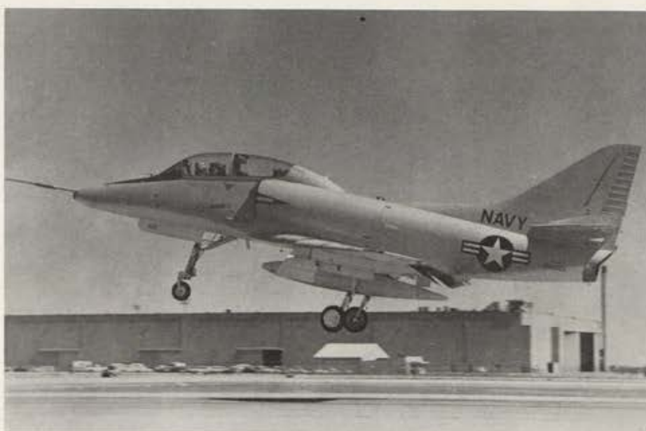
The new TA-4E, Navy-Marine Corps advanced combat trainer, made its first flight last June. It is equipped with all A-4E avionics, 5 external-stores stations capable of carrying over 9,800 pounds (4,445 kg) of ordnance, 2 20-mm cannon, Pratt & Whitney J52-8 engine, wing-lift spoilers for crosswind landings, Douglas-built zero-zero ejection seats.
