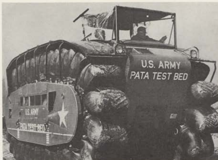
The PATA (pneumatic all-terrain amphibian), wheeled vehicle developed for the U.S. Army by Firestone Tire and Rubber Company, makes use of rotating cushions of air for support and propulsion. It is a rubber-tracked vehicle with 1.25 tons (1.13 mt) capacity. Attached to its 2 oval treads are air cells enabling it to travel over land or water.
