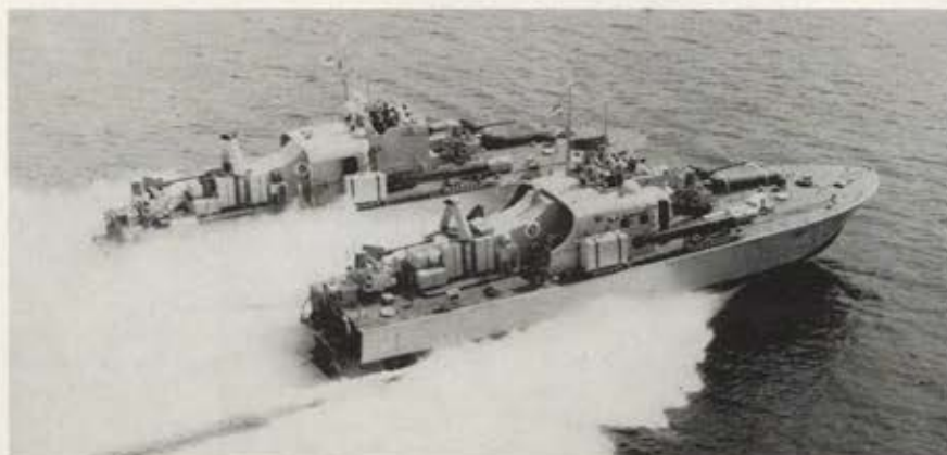
Among first vessels to employ turbine power exclusively are these British Navy BRAVE-class patrol boats, equipped with 3 Proteus engines mounted side by side. BRAVES, boasting top speed of 50 knots (92.5 km/hr), have been operational since the mid-1950s.
