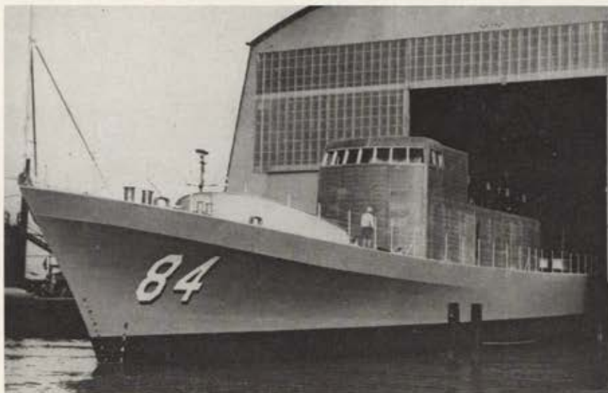
USS ASHEVILLE, shown emerging from shipyard shed in Tacoma, Washington, is one of U. S. Navy's fast new gunboats, which was to have been commissioned in December. Built of aluminum and using turbine and diesel engines, it will protect coastal shipping.
