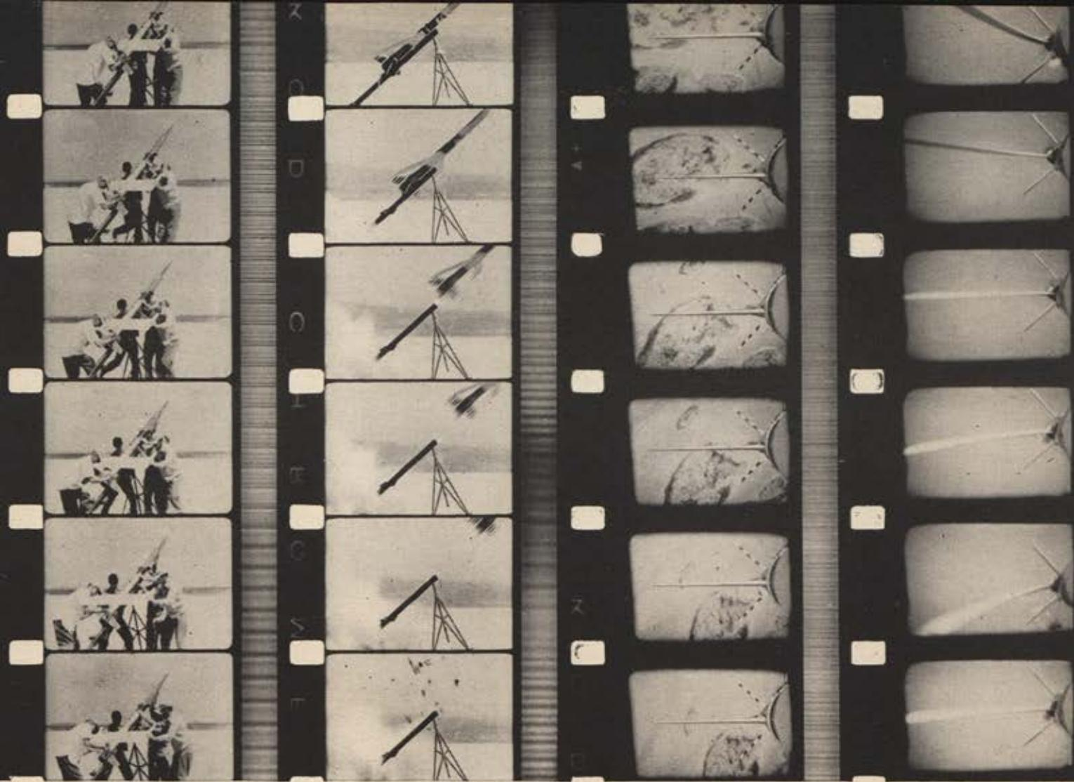
Engineers mount cameras and X-wing on supersonic rocket to test new design.
