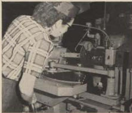
SPECIAL BALL-GRINDING machine developed by AC for grinding a ball-shaped end on a shaft to very close tolerances and extremely fine finish.
