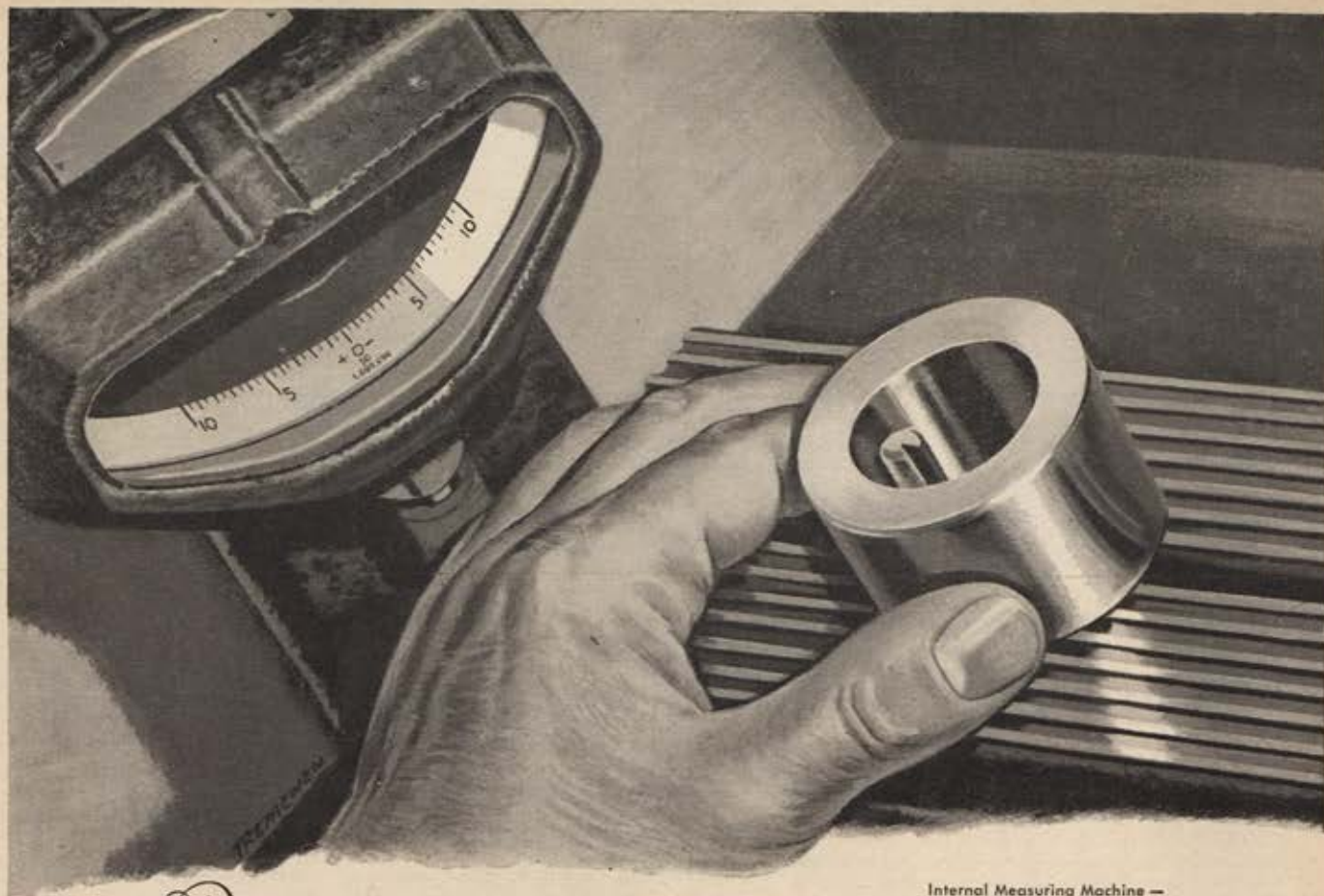
Internal Measuring Machine — capable of measuring inside diameters to a 50 millionth of an inch.
