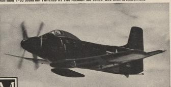
DOUGLAS A2D SKYSHARK POWERED BY ALLISON T40 TURBO-PROP
