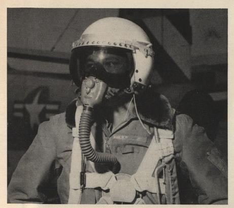
Greater safety for Air Force fighter pilots making high speed bailouts is assured with the development of a spherical visor which glues helmet to head.
