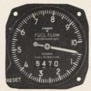
**Gravimetric Fuel Flow Totalizing Systems**
