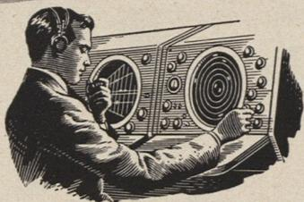
**TOWER CONSOLE** Gilfillan's desk-size, one-man GCA console is in startling contrast to the 22-ton, five-man wartime trailer. By remoting the radar data to the control tower, air traffic personnel now have accurate plane position information instantly available. Consolidation of all GCA features into a compact console is an exclusive Gilfillan improvement.
