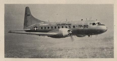
First flight picture of the Air Force's new T-29 navigational trainer, built by Consolidated Vultee is shown here. The high-speed ship, which resembles the airline's Convair Liner, is the first plane designed especially to train navigators in groups. Four astrodomes on top of the fuselage are provided for 14 students and instructors. Some of planes' 18 antennas are visible here.
