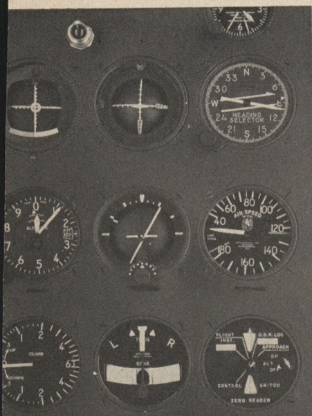
Zero Reader, top row center, shows pilot which way to move the controls.
