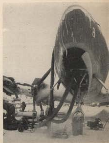
Heater ducts feed underbelly of a C-54. Hangars are used for heavy maintenance.
