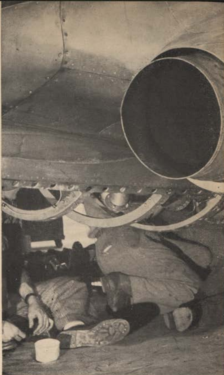
Eleven bolts hold the jet engine in place, a fact which gives most mechanics
