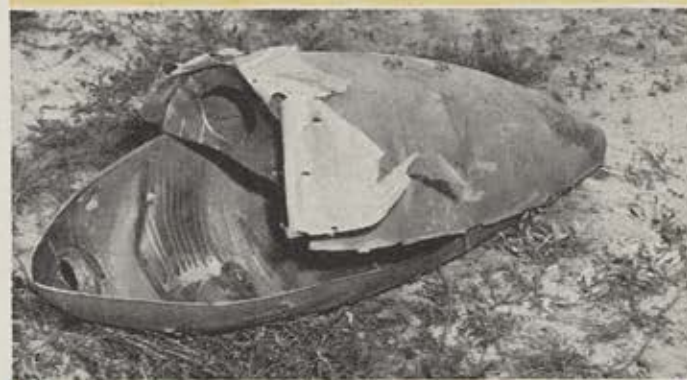
4 Metal tank, five pounds pressure. Hit by 20 mm HEI.
