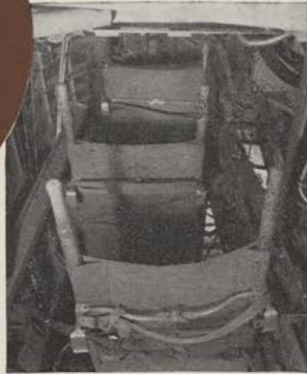
Looking up into the bomb bay of the B-17. Three litters have been slung in place with harness from field packs. Three more litters may be placed on the other side of the bomb bay.
