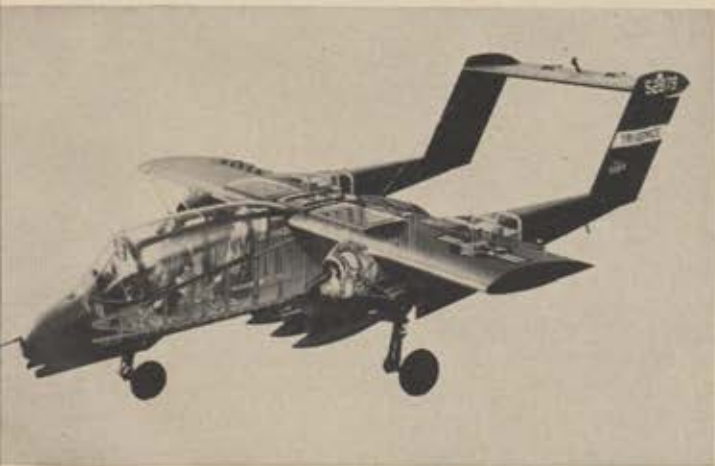
Basic layout of OV-10A is shown in this cutaway. Fuel tanks in the wing are self-sealing. The original configuration had 10 feet less wingspan. Service pilots are reportedly happy with the craft's exceptional maneuverability at low speeds and with the fine visibility the Bronco affords them.
