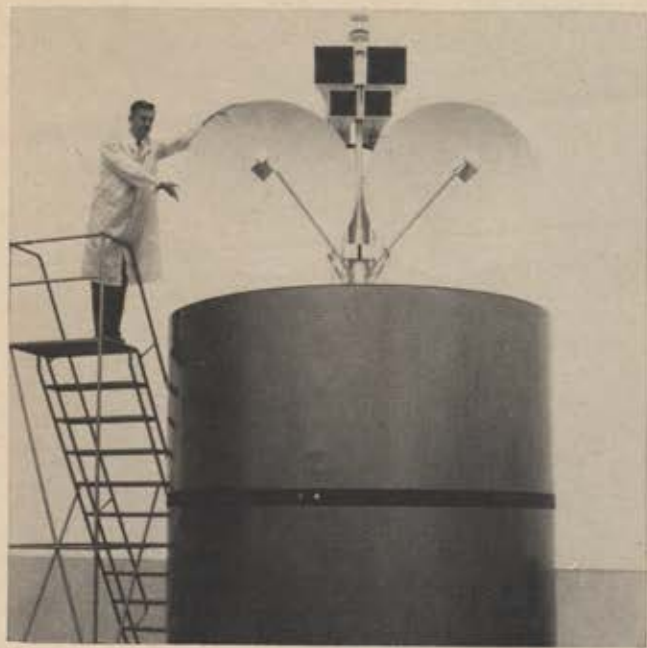
Communications Satellite Corp. has ordered huge new Intelsat-4 satellite from Hughes for service in the 1970s. Satellite will be able to handle 5,000 phone calls simultaneously.
