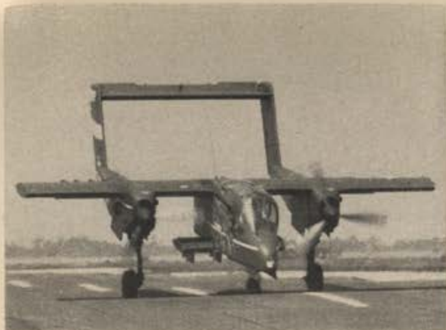
First model of the OV-10A is undergoing its rough-field landing and takeoff tests above. The special washboard strip built on top of a conventional runway is believed to provide most severe rough-field test ever given to an aircraft. It sent standard autos out of control at 13 mph.
