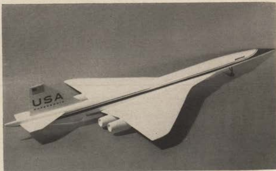
Current redesign effort of the United States supersonic transport (SST) has narrowed to one configuration, which Boeing Co. plans to submit to FAA's SST Program Office by January 15, 1969. Resembling the F-4 supersonic fighter in planform, the 2707 dash 300 design employs a fixed-wing configuration having a 50-degree sweep angle, a separate tail section, and high-lift devices.
