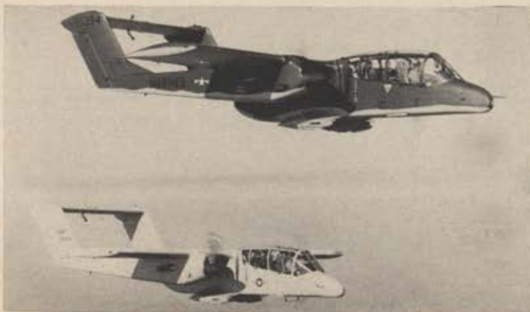
Marine and Air Force versions of the OV-10A are virtually identical, with the USAF model carrying several hundred pounds of additional communications gear. A wide variety of armament packages are available, including 7.62-mm Gatling guns, rocket packs, and bombs. Standard armament load is 2,000 lbs. for close-support and interdiction missions.
