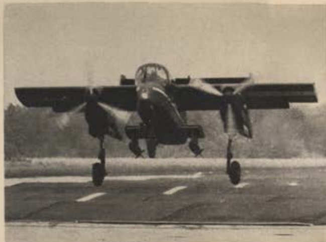
Taxi runs above 105 mph were successfully completed by the OV-10A on the washboard strip, in addition to landings and takeoffs at maximum weights. Despite its length, the aircraft's landing gear proved to be exceedingly rugged. The second model OV-10A also had no significant trouble.
