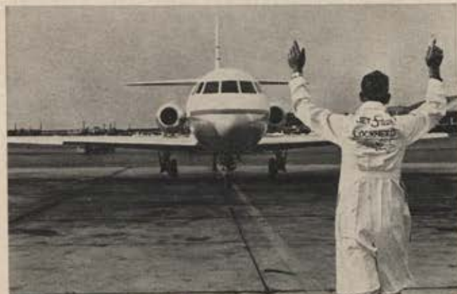
The JetStar, Lockheed's UCX jet utility transport now going into production, has reached speeds of 685 mph, altitudes of 52,000 feet, and ranges up to 3,105 miles.
