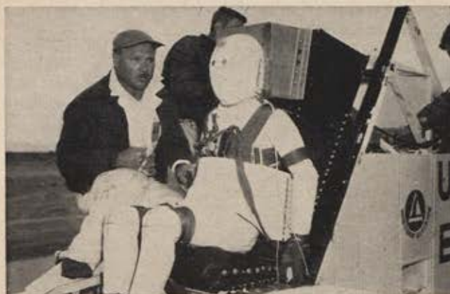
A rocket sled used to test windblast effects on a dummy clothed in a protective suit hurtled to almost Mach 2, 1,200 mph, at ARDC's Holloman AFB, N.M. The AF later revealed that the rocket vehicle has reached 2,853 mph.
