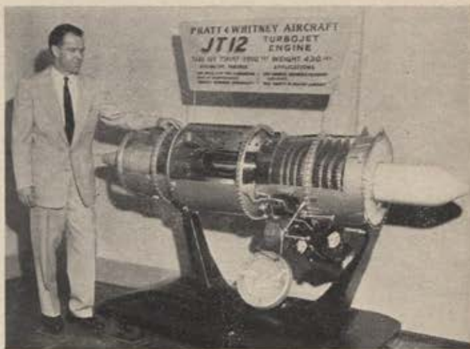
JT12 JET ENGINE, the smallest built by Pratt & Whitney Aircraft, produces 2900 pounds of thrust for a total weight of only 430 lbs. With a single spool and fixed geometry, the JT12 promises outstanding performance, reliability and ease of maintenance for many possible applications.
