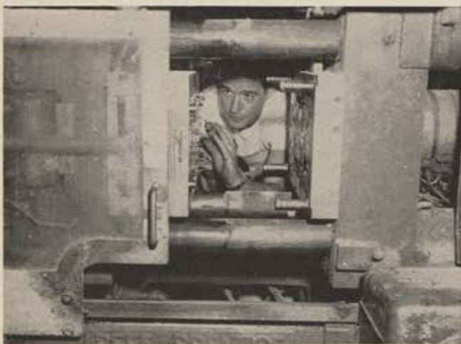
When steel mold is finished, it is placed into injection molding machine into which plastic is poured for production.
