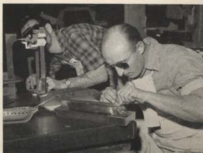
After handmade model is approved, steel molds are cut. This moldmaker duo is inspecting Revell ship model.
