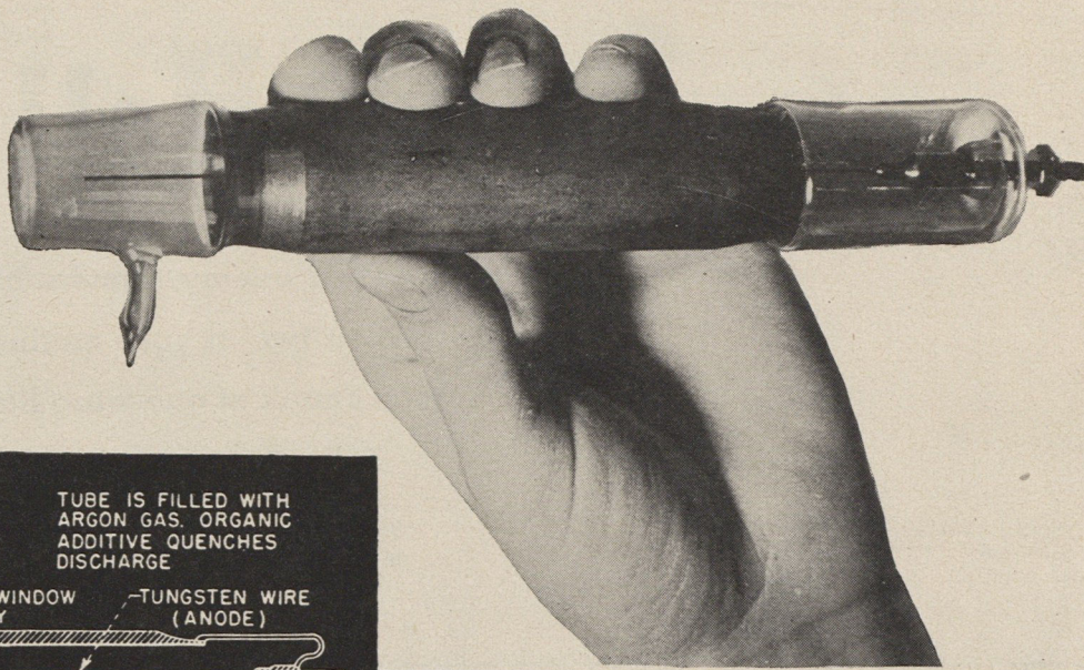
Sectional of a Geiger tube, showing how ionization triggers the electronic circuit. Above, a typical detector tube, from a portable counter outfit.
