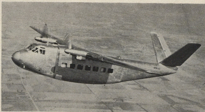
Beechcraft's new Twin-quad twenty-place short-haul transport features the “butterfly tail” used on the Bonanza, and a unitwin power system using two opposed engines buried in the wing. In case of power failure, either engine can turn the propeller.
