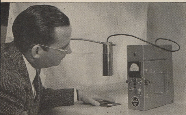
Portable Geiger Counters are in commercial production and have varied uses. Here a detector unit is used to test mineral samples for traces of radioactive content.
