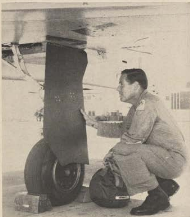
Landing gear door made of aluminum honeycomb core covered with bonded layers of boron composite skins has been tested at supersonic speeds on this F-5 fighter. Northrop, which developed structure, says the strong yet lightweight material could be used to build complete airframes.
