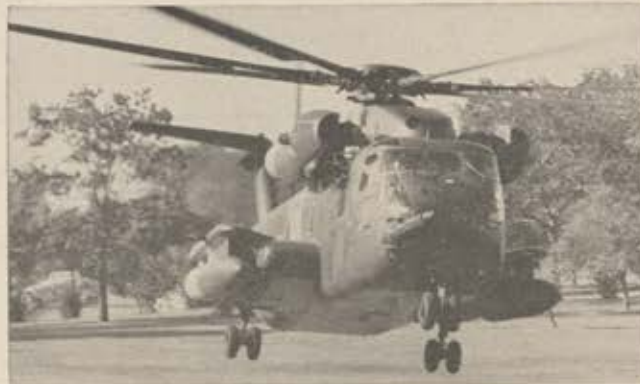
Hovering, the HH-53C points its refueling probe almost directly at camera. The 20,000-pound external hook for raising cargo could accommodate an entire Apollo spacecraft.
