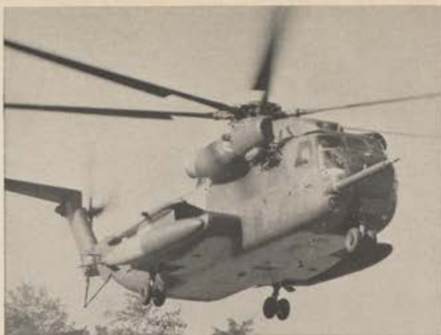
Airborne shot of the HH-53C provides good view of the auxiliary fuel tanks. These come in two sizes, can carry 450 or 650 gallons and withstand incendiary shell hits.
