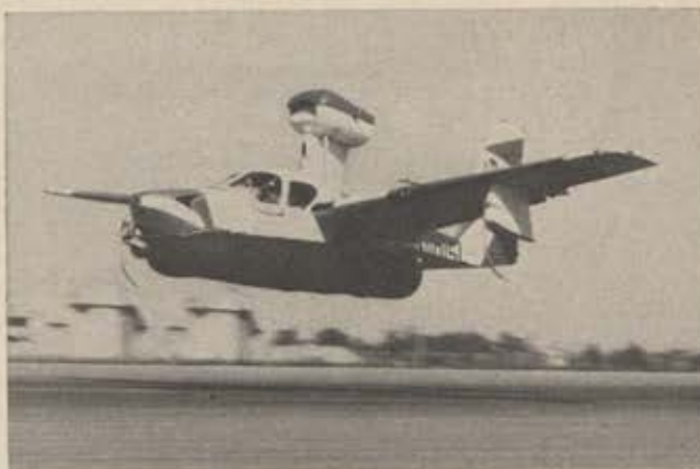
Air cushion landing gear (ACLG) developed by Bell Aero-systems Company, Buffalo, N. Y., is tested on LA-4 Lake amphibian testbed. Unique gear, dotted with tiny nozzles, forces out layer of air enabling plane to "float" to landing on water, swampland, gravel, or other unimproved surfaces.
