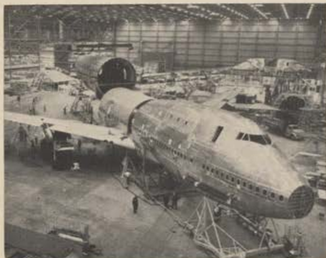
With forward fuselage in position and wings and center section now in place, the aft-fuselage section of the airplane is positioned, loosely aligned with the remaining sections.
