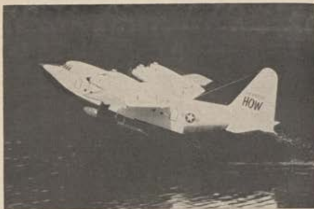
Radio-controlled six-foot-long model of Lockheed C-130 Hercules, built by Lanier Industries of Gainesville, Ga., takes off from north Georgia lake during tests for US Navy Air Systems Command, studying feasibility of employing 175,000-pound propjet Hercules in amphibious operations.
