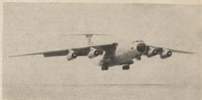
Though designed to land only on paved runways, Lockheed C-141 StarLifter is shown here in limited test of operating from bare soil at Harpers Dry Lake near Edwards AFB, Calif. After feasibility studies on aluminum mat surfaces at Dyess AFB, Tex., extensive bare soil tests are being proposed.
