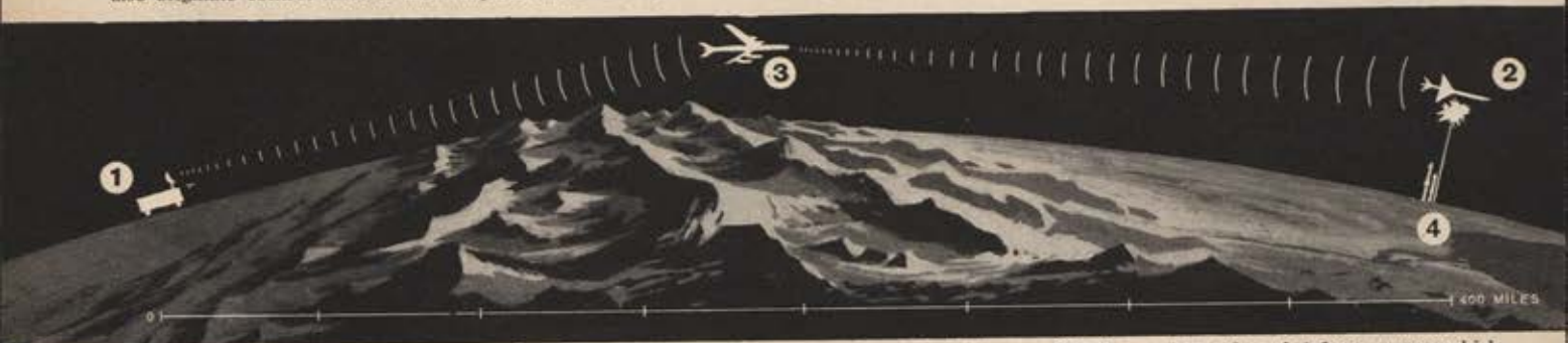
GREAT RANGE of Sperry microwave command guidance system is shown in diagram. Ground station (1) controls target drone (2) either directly
