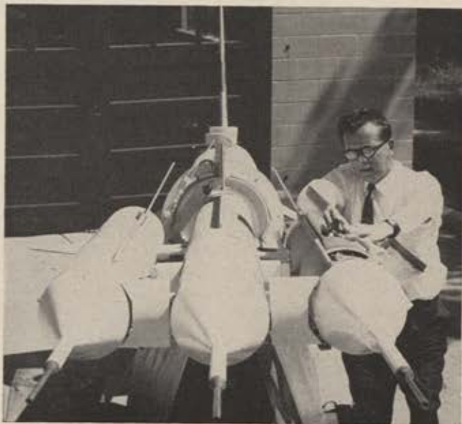
A supersonic parachute-testing rocket, the Cree, has been developed by ARDC's WADC, Dayton, Ohio. The unit can test three parachutes simultaneously, at altitudes from 30,000-50,000 feet and speeds from 1,520 to 3,040 mph.
