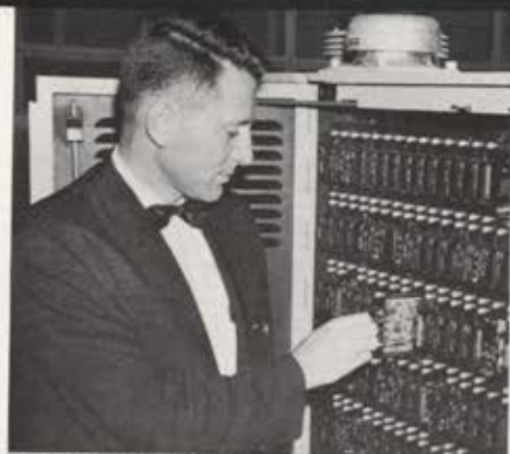
Launching and control order computers for TARTAR Missiles. Electronic and electromechanical portions of this all-transistorized modular computer are shown at left and right.
