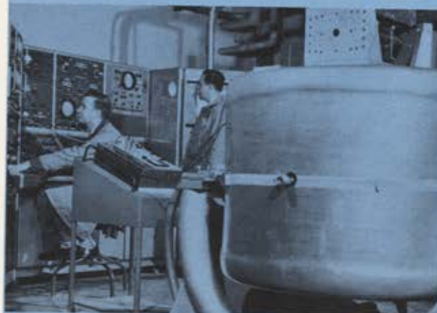
Vibration testing of missile component. Such tests duplicate inflight environments that components undergo when missiles are fired.
