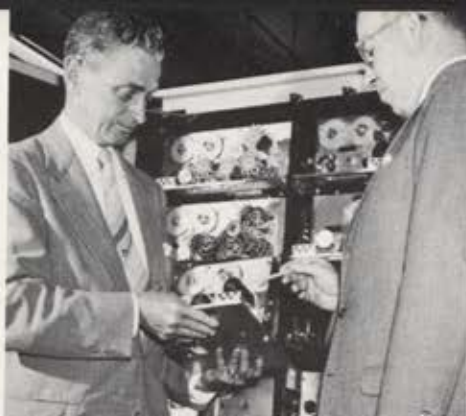
Launching and control order computers for TARTAR Missiles. Electronic and electromechanical portions of this all-transistorized modular computer are shown at left and right.
