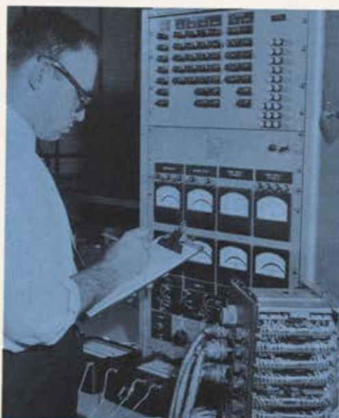
Missile-borne computers. Ford Instrument computer experience covers every phase of ballistic missile guidance and control. Typical is this control computer, shown during test, for U. S. Army JUPITER.
