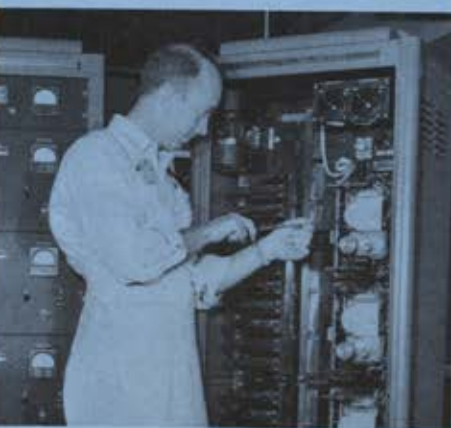
Ground support equipment. Here pre-launch computer undergoes final adjustment. Modular techniques enabled this unit to be produced and delivered in less than 6 months.
