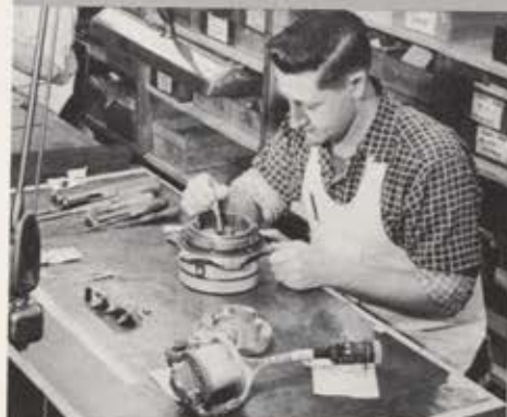
Actuators for jet vanes, air control-surfaces. This rotary actuator is driven by 1 hp d-c servo motor (shown in foreground with cable attached). Both motor and actuator are made by Ford Instrument.
