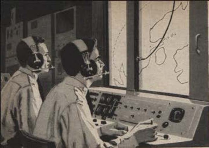
GROUND CONTROL of target drone centers in air-portable van. Men at console maintain control through flight instruments. Path of drone is traced automatically on plotting board at right.
