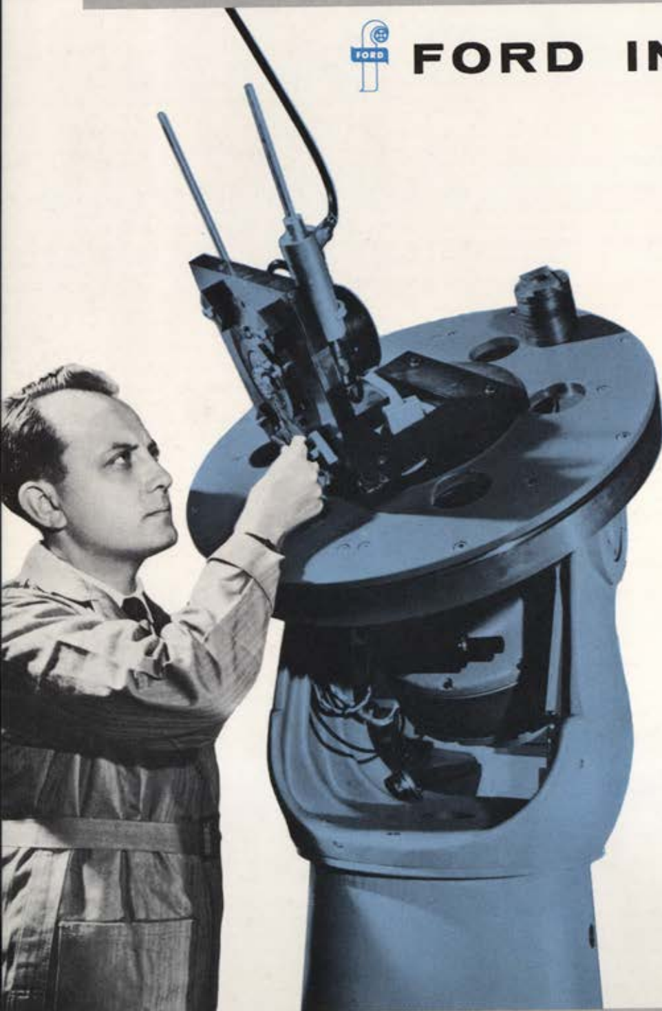
Equatorial test stand, built by Ford Instrument for its own laboratory facilities, is used for conducting basic drift error research. This type of unit can also be built to contractor order.
