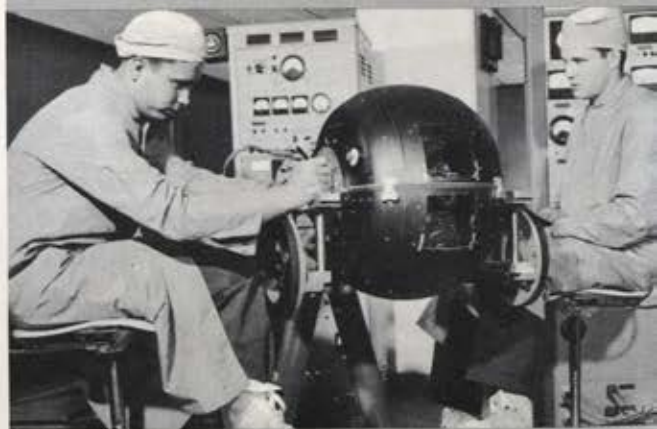
Stable platforms. Technicians here are performing test operations on a stable platform for the U. S. Army JUPITER Missile; these platforms are in quantity production at Ford Instrument.
