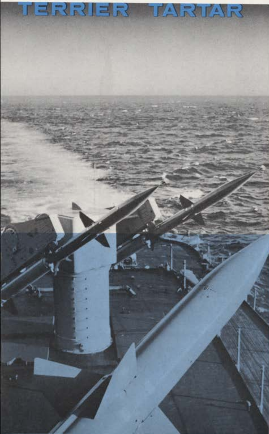
TERRIER Missiles on U.S.S. Boston. Ford Instrument-built computers solve launching and control order problems for this beam-riding missile. U. S. Navy Photo.
