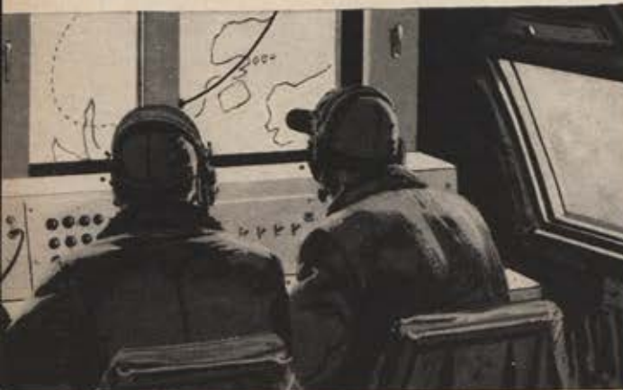
AIR CONTROL relays commands from ground station to drone where distance or terrain block direct beam. Air director may also originate control since it has complete microwave system.
