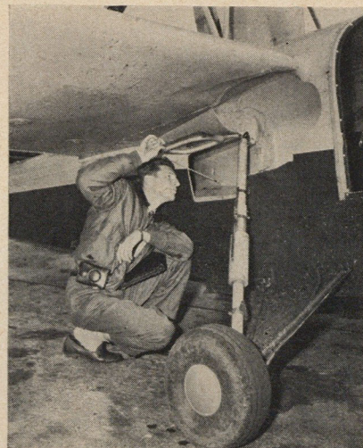
Hugh M. Pierce checks landing gear on the GA-2, noting how neatly the wheel will fit into wing root as the strut moves upward and to the rear.
