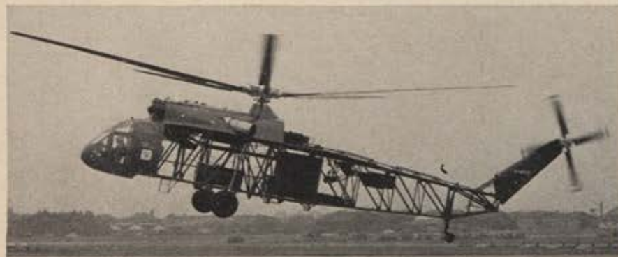
On exhibition was Britain's largest private-venture helicopter, the Westland Westminster. Picture shows the craft taking off rearward. A kind of flying crane, the Westminster is under development as a forty-eight-seat transport.
