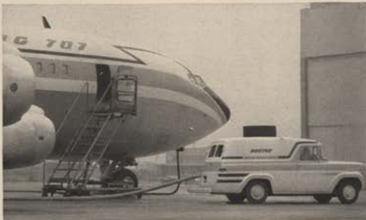
JET-GIANT STARTER. Powered by Boeing 502 gas turbine compressor, Turbo-Starter in truck provides fast, sure starts for jetliner and jet-bomber engines, and supplies air for ground operation of pneumatic systems. Other Boeing 502-series gas turbines power aircraft, boats and generators for the U.S. Navy and industrial concerns.
