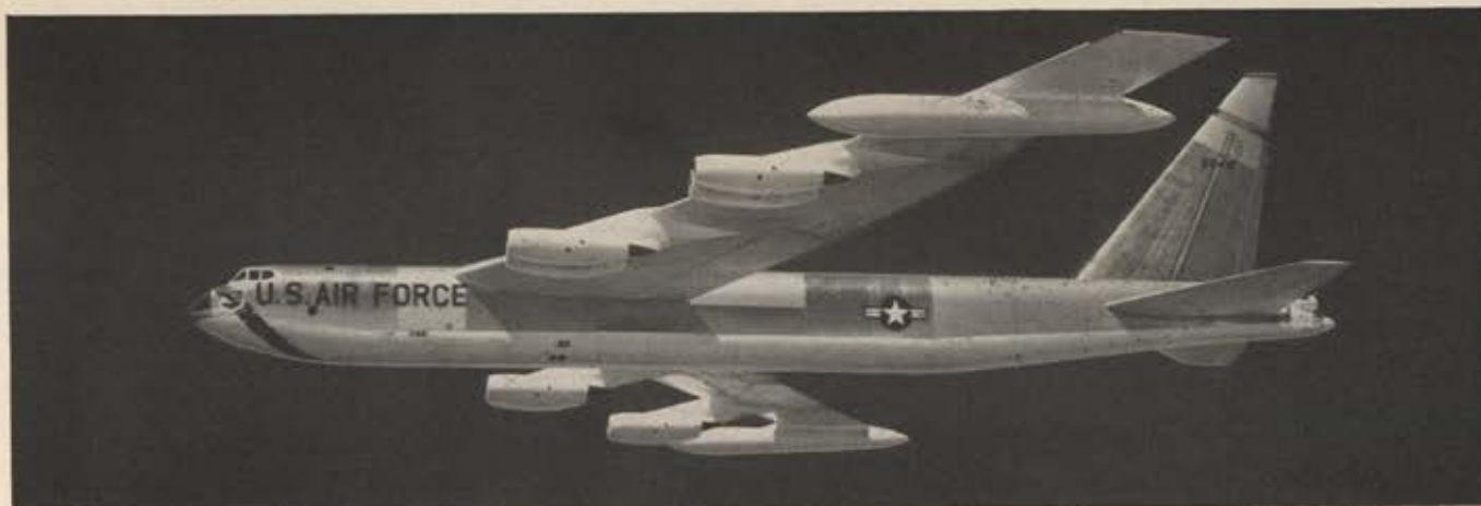
WINGED MISSILE PLATFORM. Boeing B-52 global jet bomber is Strategic Air Command's principal long-range retaliatory defense weapon. Advanced model will carry two supersonic air-to-ground missiles in addition to nuclear bomb load, combining accurate long-range guidance with supersonic weapons delivery. New B-52 will be able to destroy several targets thousands of miles apart on a single retaliatory mission.
