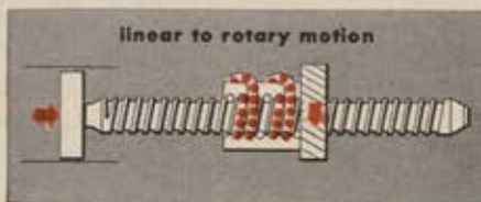
SCREW TRAVELS: When rotary motion is applied to the b/b nut, the screw glides along its longitudinal axis on rolling steel balls, converting rotary force and motion to linear force and motion with unprecedented efficiency.
