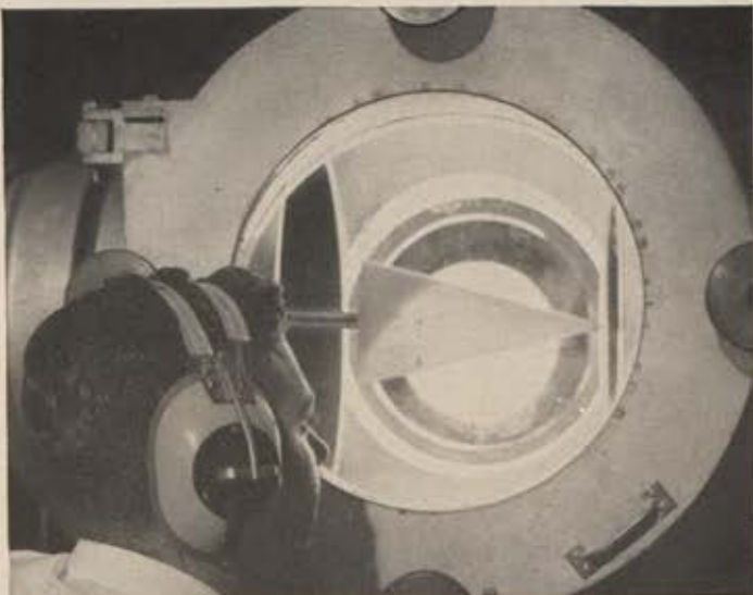
BIG WIND. Boeing's hypersonic wind tunnel tests models at speeds from five to eight times that of sound. Research programs at Boeing cover all fields of space-age technology. Development projects include Dyna-Soar, a manned space vehicle that will orbit at speeds approaching 18,000 miles an hour and be capable of re-entry and normal landing.
