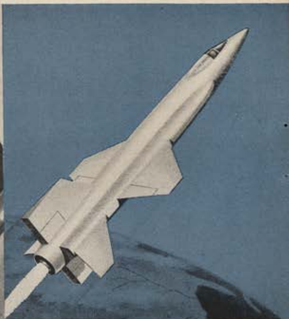
HYPERSONIC, ROCKET-POWERED X-15 manned research aircraft by North American is designed to explore near space. Sperry inertial system, developed for USAF, will give pilot data for navigating and maneuvering the NACA-sponsored X-15 with extreme accuracy at speeds of one mile per second.
