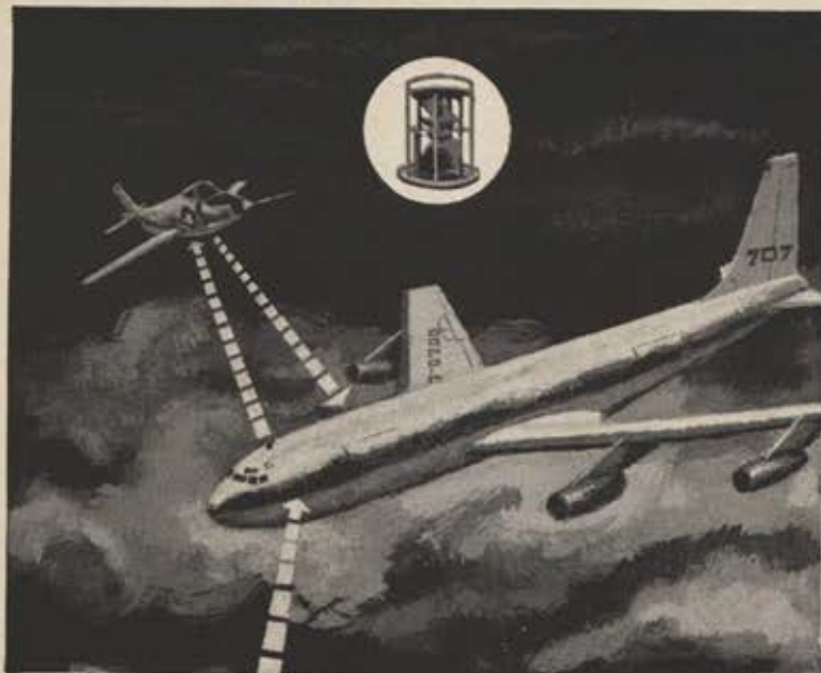
Aircraft Proximity Warning System utilizes modulated beams of light to detect the approach of aircraft from any direction as far away as 5 to 7 miles.
