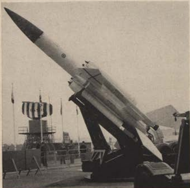
On display in the guided-weapon park was the Bristol Bloodhound surface-to-air missile. Bloodhound has two Bristol Thor ramjets for sustainers, is to be used in home defense.
