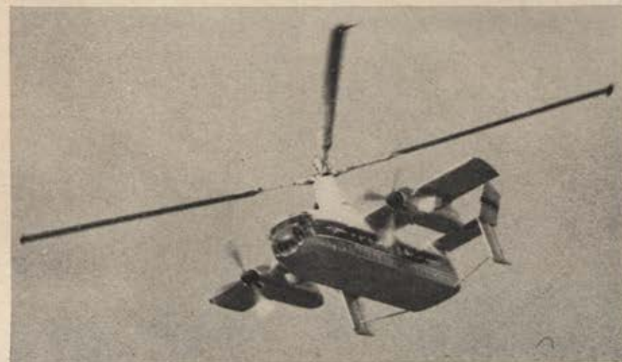
Considered by many the most radical plane at the show was the Fairey Rotodyne VTOL transport, a forty-eight-passenger craft with military, civil applications.
